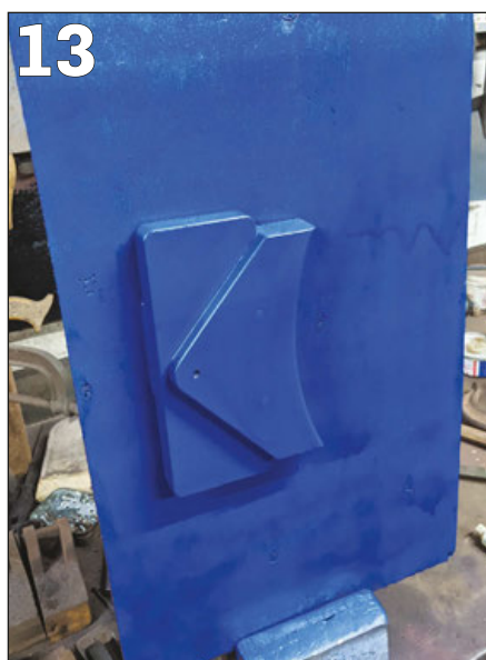
PHOTO 11: 3D printed two-part pattern for new brake blocks, complete with locating holes.
