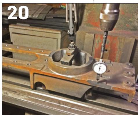
horn guides. The setup process for these was very similar to that for the horn blocks, with a bit of white paint and some careful measuring being used to set the castings up true to the bed of the mill.
