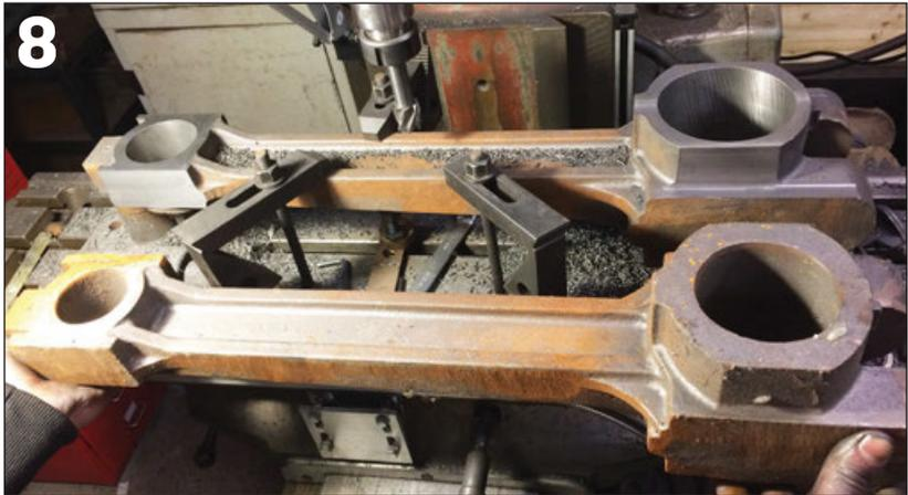
**PHOTO 09-10:** Block flipped to machine down rear side to finished width.
