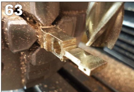
the lathe and part off (Photo 61). It's worth pointing out an important but not obvious function of the pan-headed screw that holds the eccentric to the crankshaft, the head of this screws retains the outer eccentric arm on the eccentric whilst allowing it to rotate freely.
