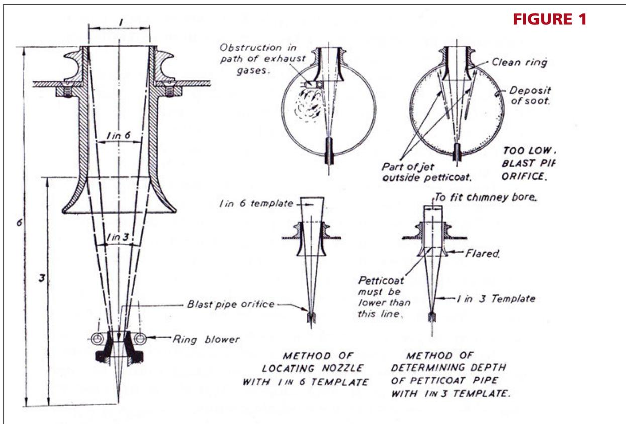
There are two types of chimneys: a) those of a constant diameter from top to bottom and b) a chimney with a tapered bore. A tapered chimney works better than a parallel one as it has a venturi effect at the top of the
