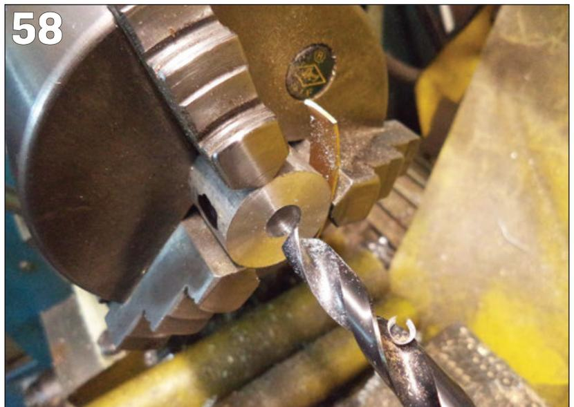
have to use a parting tool (**Photo 59**). Remove from the bush, re-chuck the bar and turn down a small spigot but leave a reasonable thickness for
