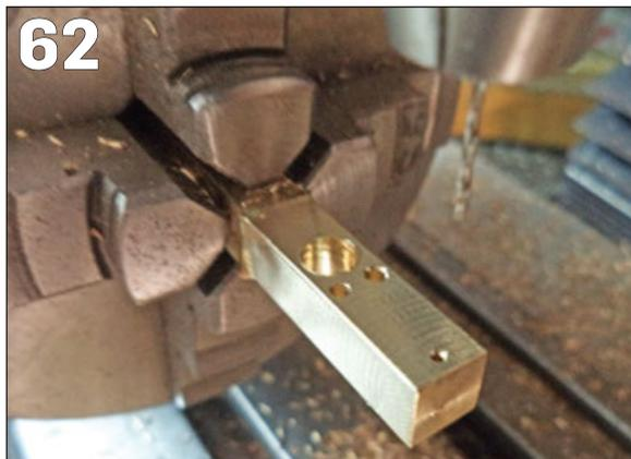
“The flat nose of the grub screw will pull the bar into the correct orientation...”
