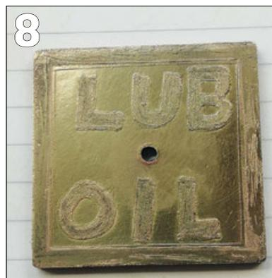
use as some table and cooking salts also contain other chemicals. It's also recommended that you use de-ionised water, the sort you top up your car battery with or use in a steam iron. For my experiments I used tap water which worked perfectly.
