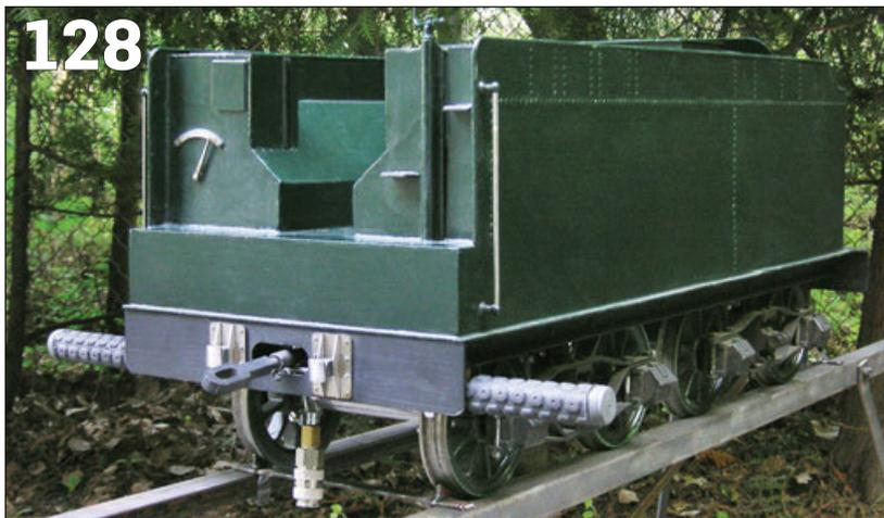
**PHOTO 128:** Front end of tender. Note the rubber foot rests.
