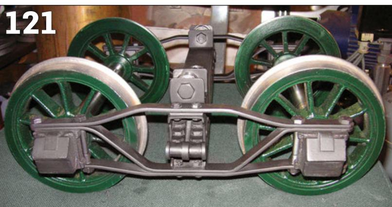
bogie bolsters, at the arrows in **Photo 120**, ensure frictionless rotation of the bogies around their kingpins. The bogie frame is very simply constructed of narrow flat iron strips bent to shape. A rectangular steel tube functions as bolster. A hole drilled in the tube accommodates the king pin, a piece of 16mm axle steel which is firmly attached to the tender frame.
