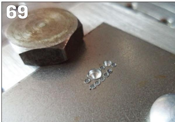
**Sketch 4** I drilled out the basic shape and then using a 1mm slot drill generated out the curves of the quadrant (Photo 69-70). It was then just a matter of joining up the dots with Swiss files to complete the overall profile (Photo 71).
