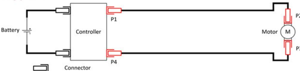
think and can develop relatively rapidly. A little corrosion on a connector will increase resistance. This increased resistance will generate heat which will speed up the corrosion process (it being a chemical reaction), as highlighted earlier. If the loco is used regularly and stored in a damp environment (does anyone put their electric loco on the mantelpiece?), this may well become an issue over time.
