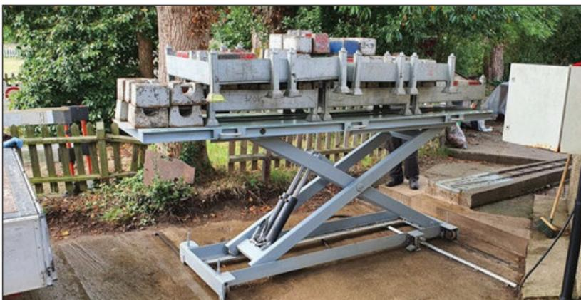
**LEFT:** Here comes the heavyweight contender – Rugby ME's new loco lift undergoes a weighty test.
