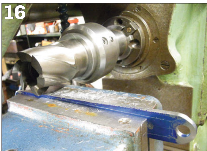
PHOTO 14: Boring the stainless steel power cylinder....
