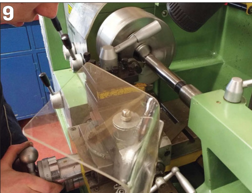
PHOTO 7: Drilling the opposing holes in the new brass flywheel.
