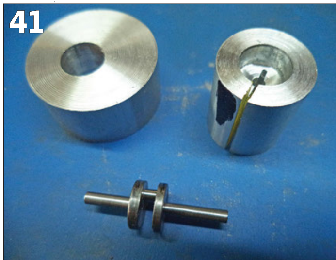
PHOTO 41: Turned one-piece crankshaft with both fixtures.
