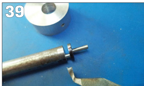
PHOTO 37: Turning the crankshaft down to 2.5mm.
