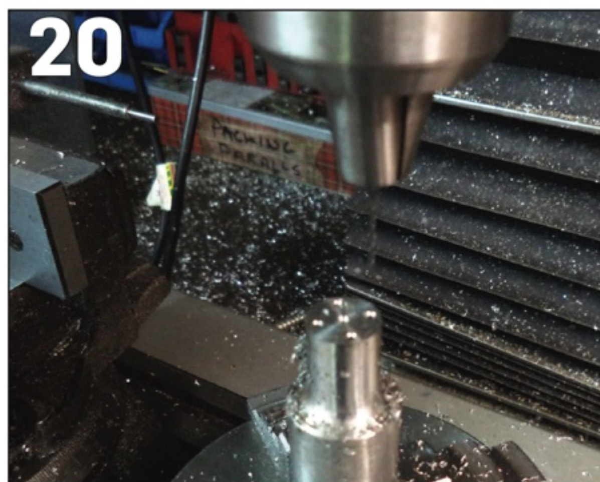
PHOTO 18: End mill used to shape outside of base.
