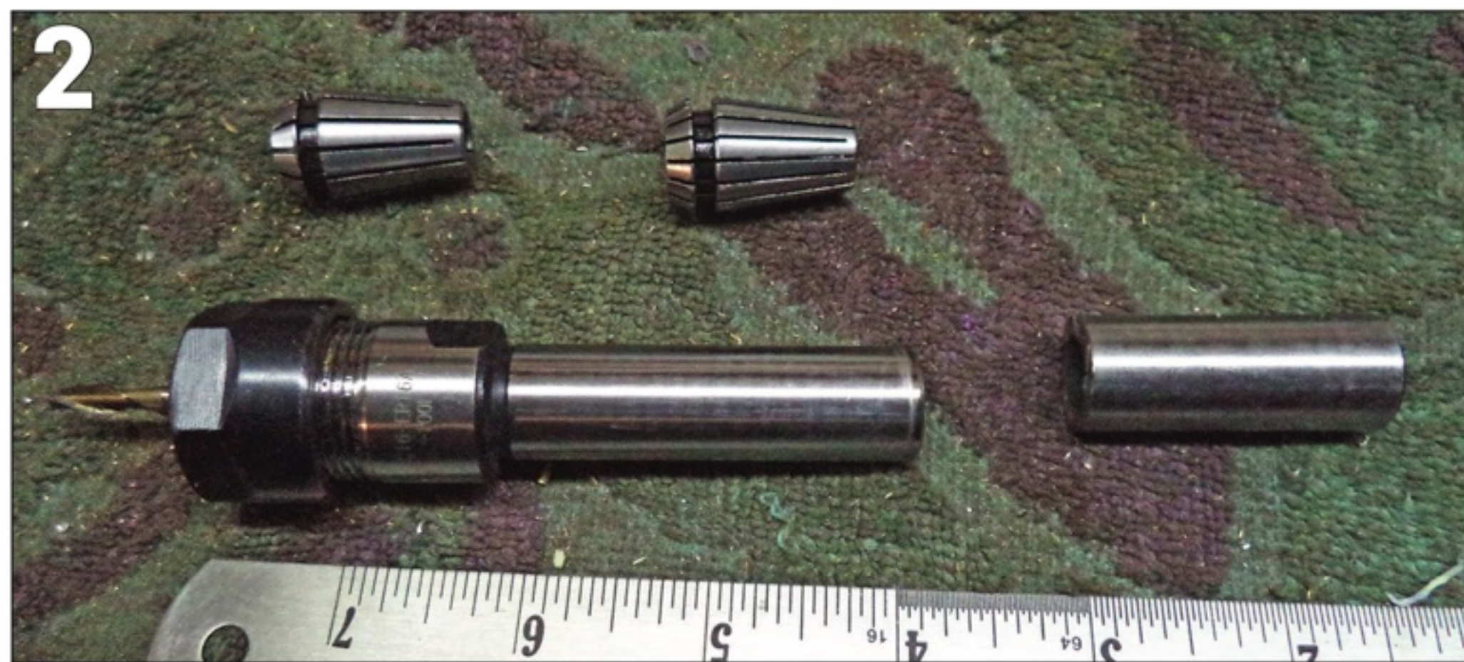
PHOTO 3: ER16 straight shank collet holder in ER32 collet to fit mill.
