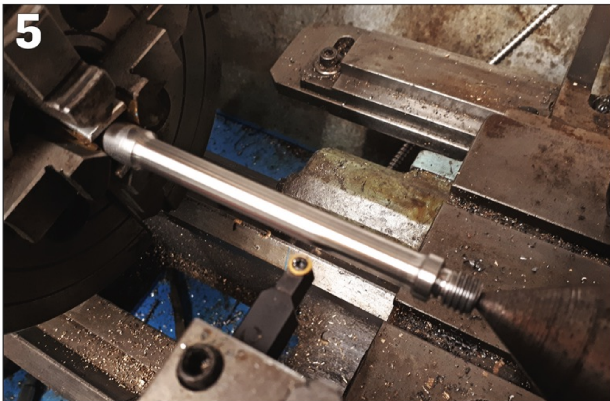
PHOTO 4: Finishing the hammer head.
