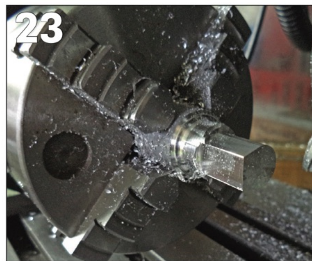
PHOTO 26: Cylinder drilled and reamed 6mm.
