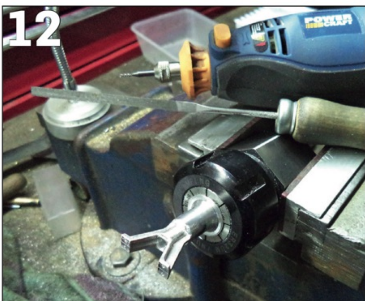
PHOTO 10: Finishing sides of cylinder stand.
