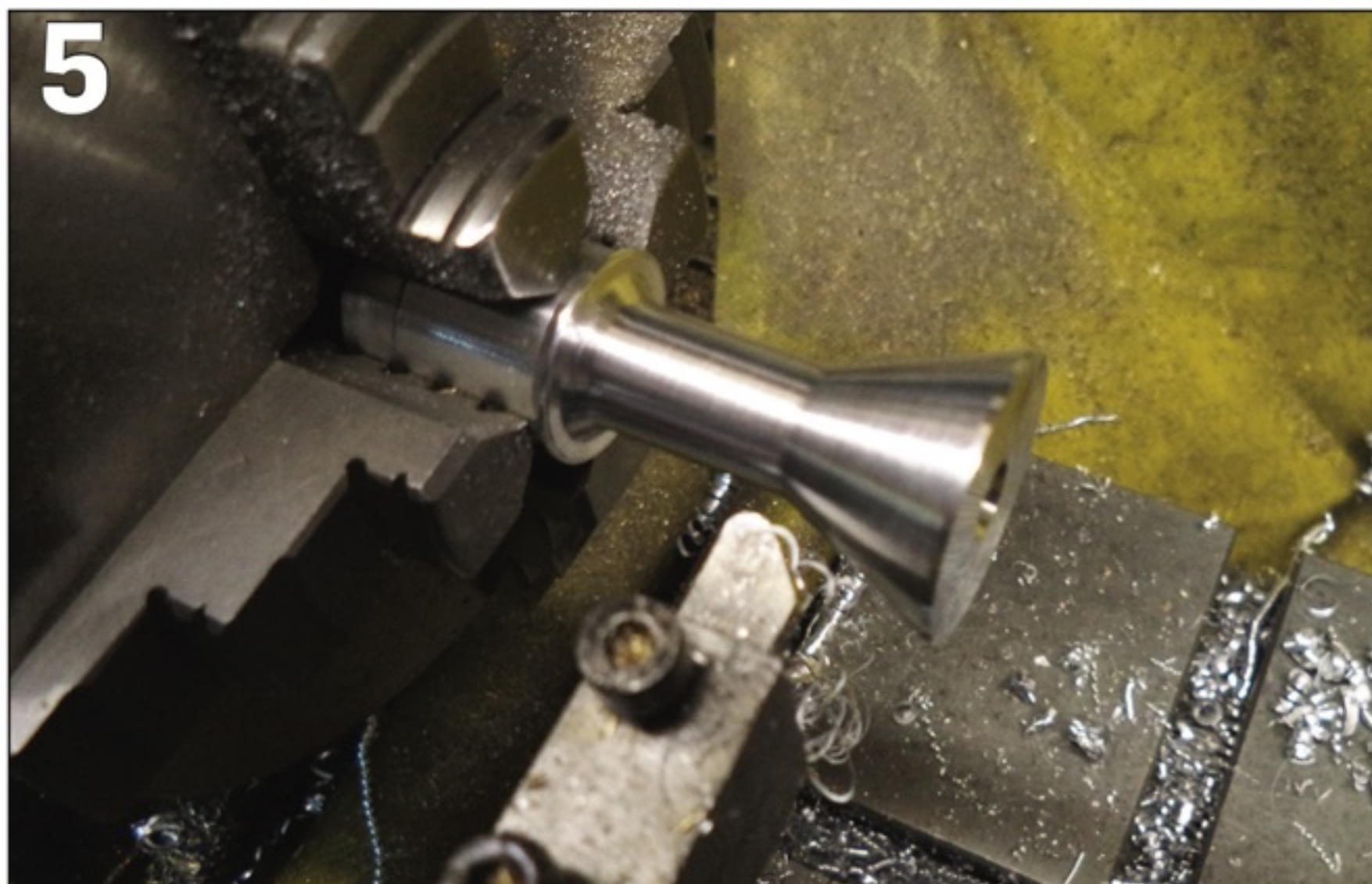
PHOTO 5: Machining out cone of the cylinder stand.
