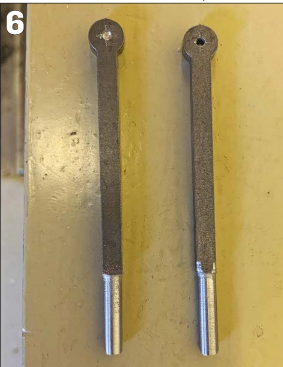
PHOTO 6: Step 1 complete – turned shaft ends from setup in Photo 5.
