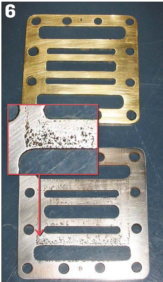
PHOTO 6: Severely corroded steel port face plate, lower, brass replacement, upper.
