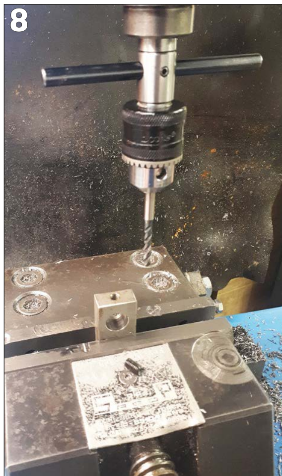
PHOTO 7: Material for arm set in vice on parallels before being drilled and reamed.
