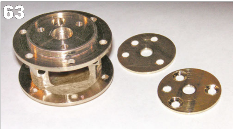
PHOTO 61: The cylinder and the port face block are tinned with soft solder.
