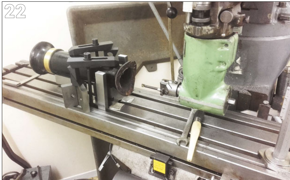
PHOTO 22: The chimney casting being bored out for spark arrestor.
