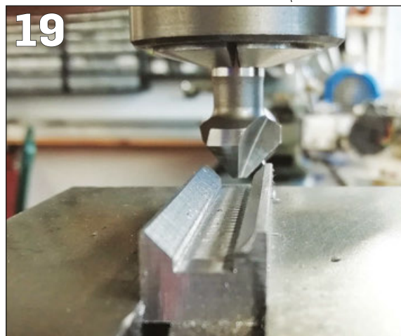
PHOTO 19: Angle machined with countersink.
