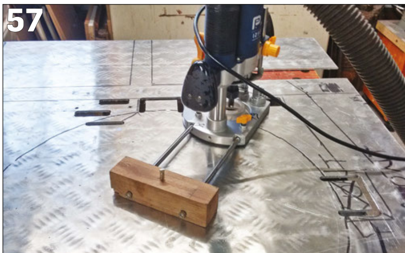
PHOTO 57: Wood router used to cut hole in cab plate for boiler.
