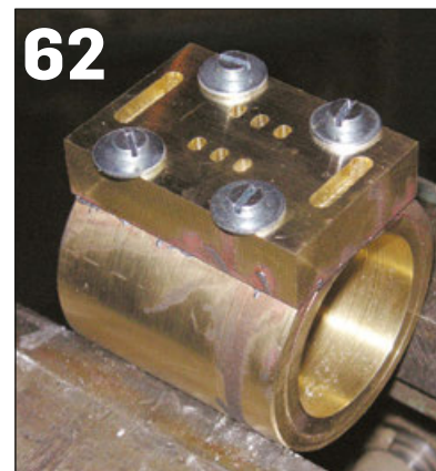
PHOTO 62: Screws are tightened while assembly is hot.
