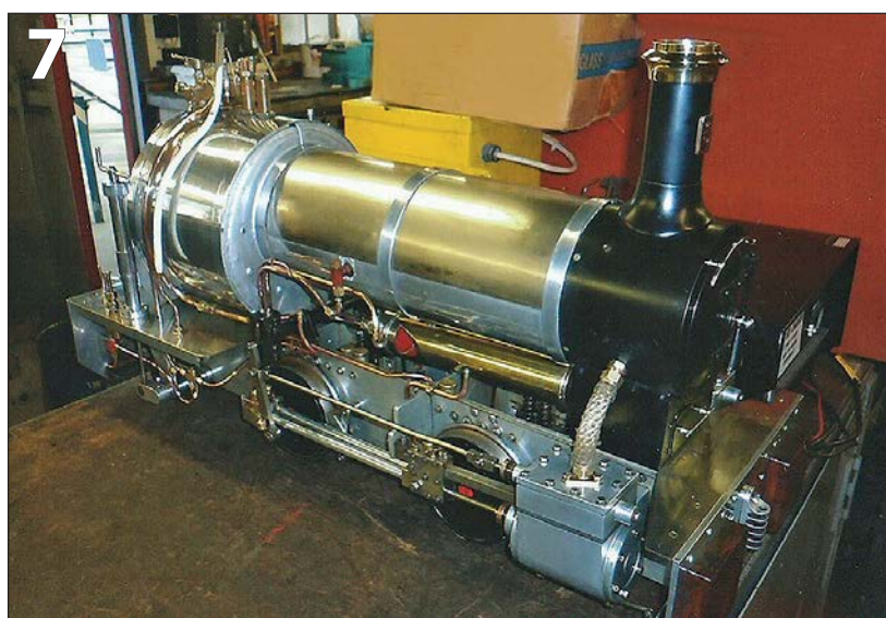
PHOTO 7: Alicat without cab and saddle tank – the 8-inch long x 1\frac{1}{2} -inch diameter whistle and blower pipe are clearly visible. Note saddle tank water gauge, painted white, one side only, to right of the handbrake stanchion and left of the steam turret.
