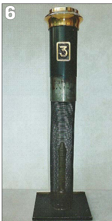
PHOTO 6: Spark arrestor, smokebox, baseplate, and chimney assembly.
