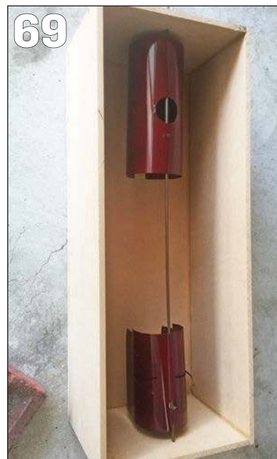
PHOTO 69: Baking cabinet made from sheets of MDF.
