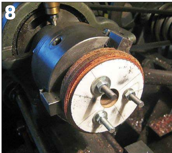
PHOTO 8: The flywheel jig mounted on the lathe.
