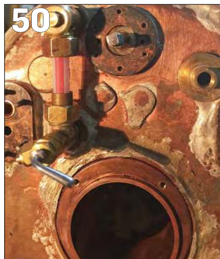
PHOTO 53: Fly-cutting saddle for the smokebox...
