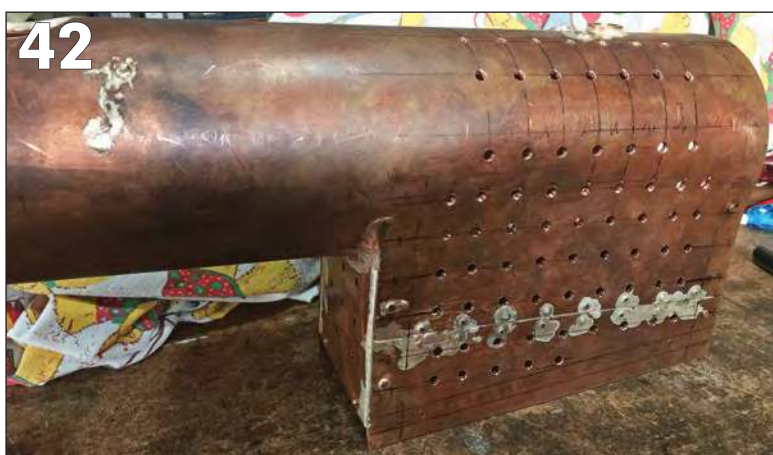
PHOTO 38: Checking position of inner firebox to outer wrapper with a spacer.
