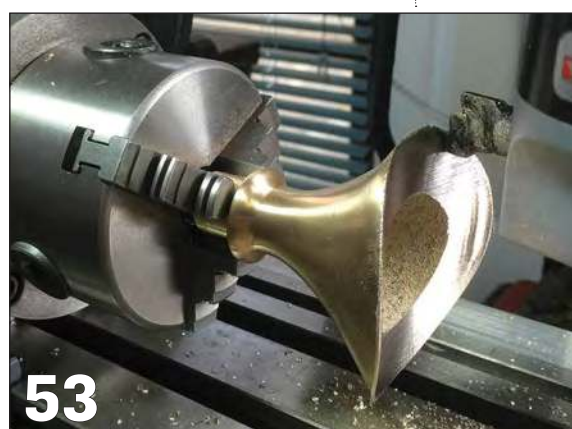
PHOTO 55: Boring out the chimney proved a challenging job.
