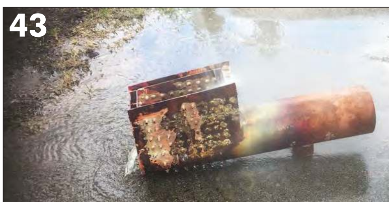
PHOTO 43: Soldering up the boiler – a long drawn-out and repetitive process.
