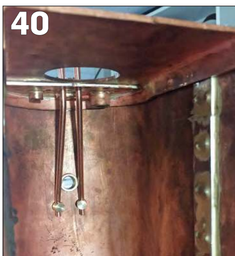
PHOTO 38: Checking position of inner firebox to outer wrapper with a spacer.
