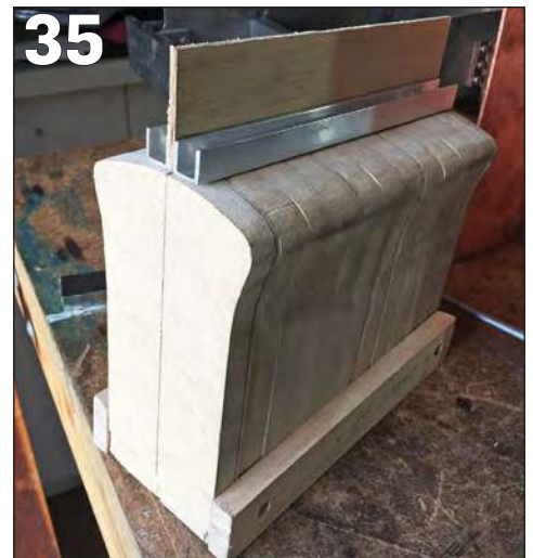
PHOTO 32-37: Stages in forming the firebox outer wrapper and inner firebox.
