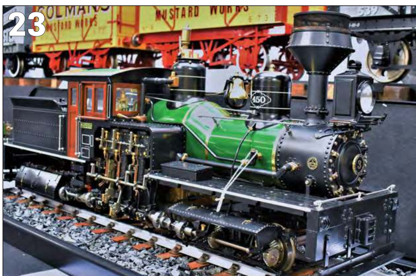
PHOTO 23: A superb example of a 3-cylinder Shay logging locomotive in 5-inch gauge by Stewart Jackson.
