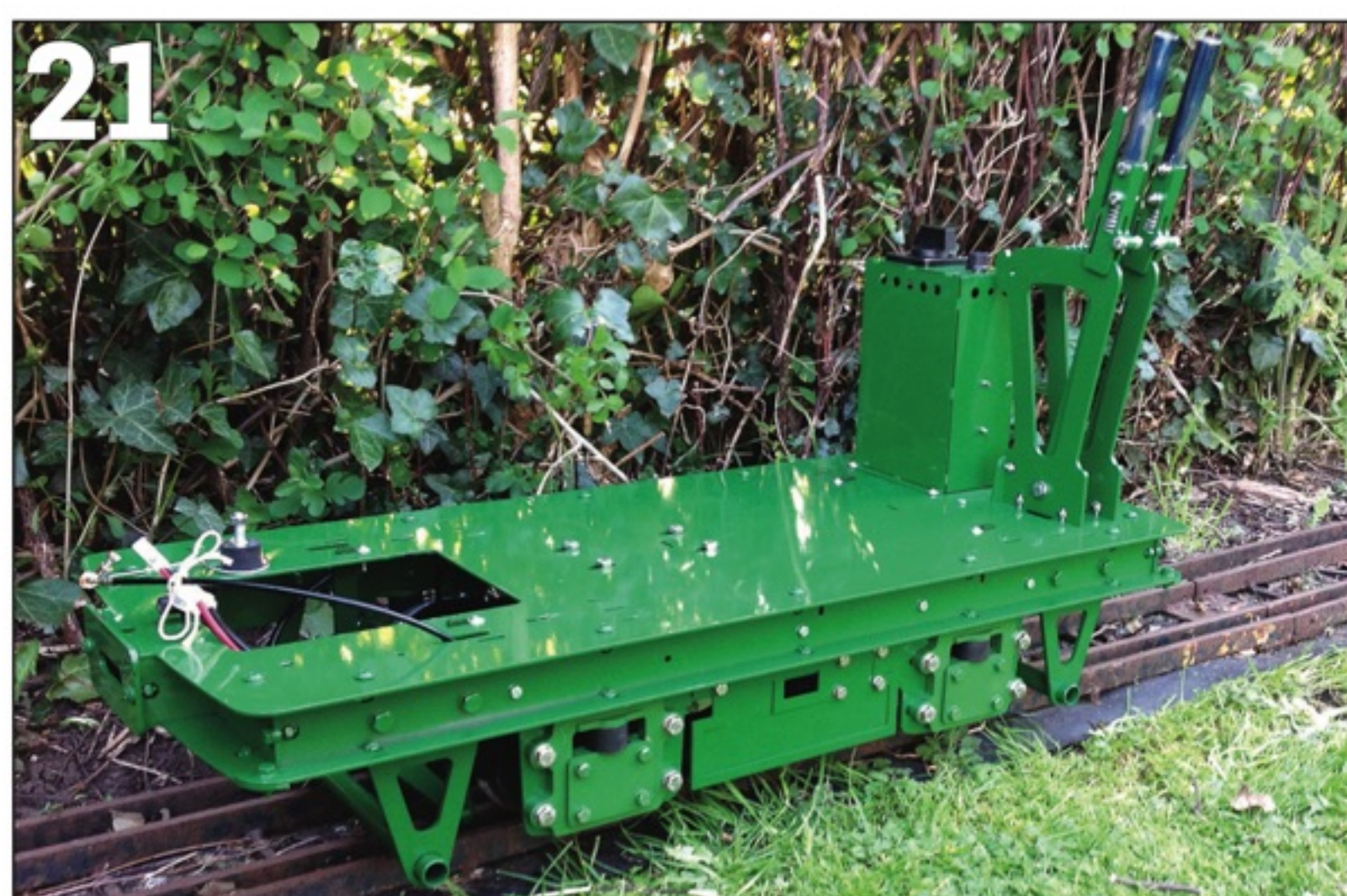
PHOTO 21: The frame ready to be loaded into the car. The square hole at the front is where the generator drops in with the motor above the frame, covered by the bonnet. The seat slots into holes in the frame to the left of the control levers. One lever engages the drive from the motor to the generator, the other is a powerful handbrake.
