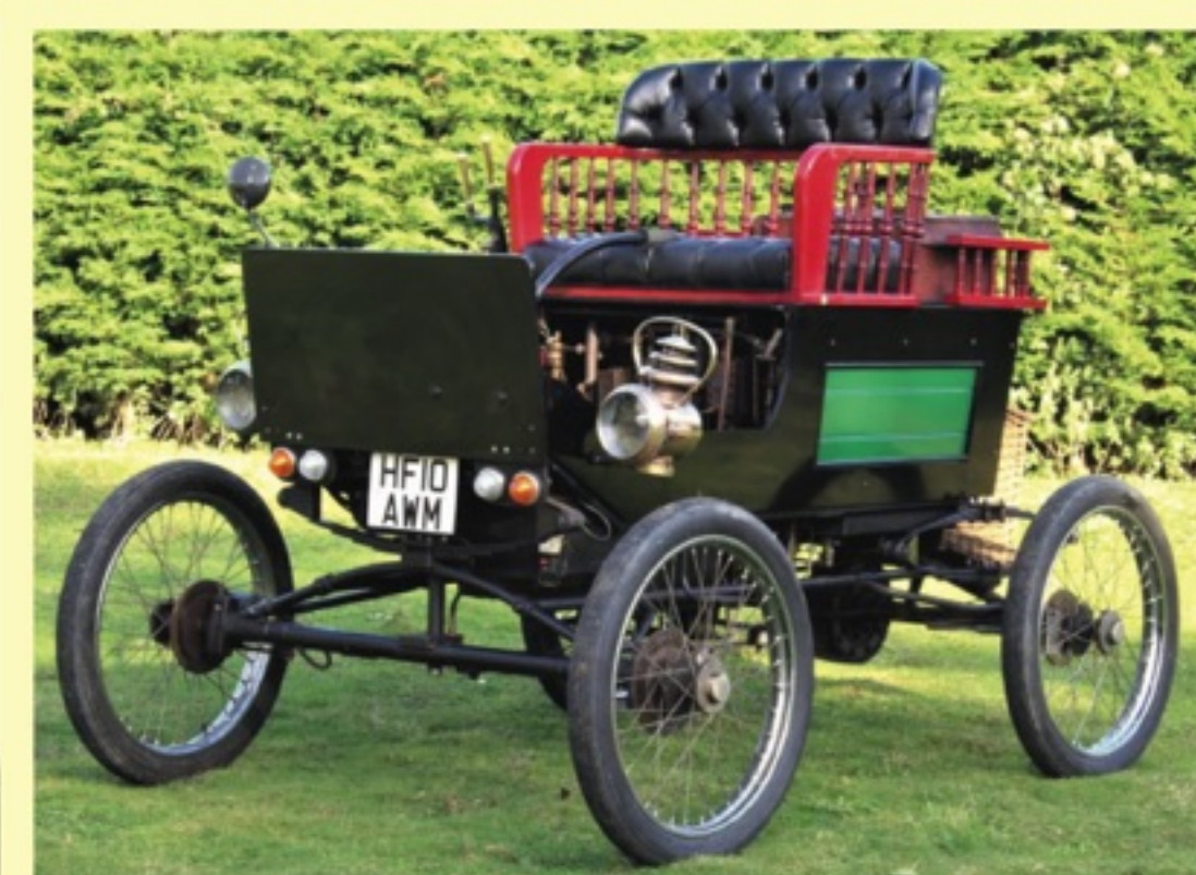
LIKAMOBILE STEAM CAR Running on heating oil, the boiler steams from cold in ten minutes. It's been in regular use and has been fitted running lights and indicators back and front. Complete with a commercially built lightweight road trailer. £14,750
