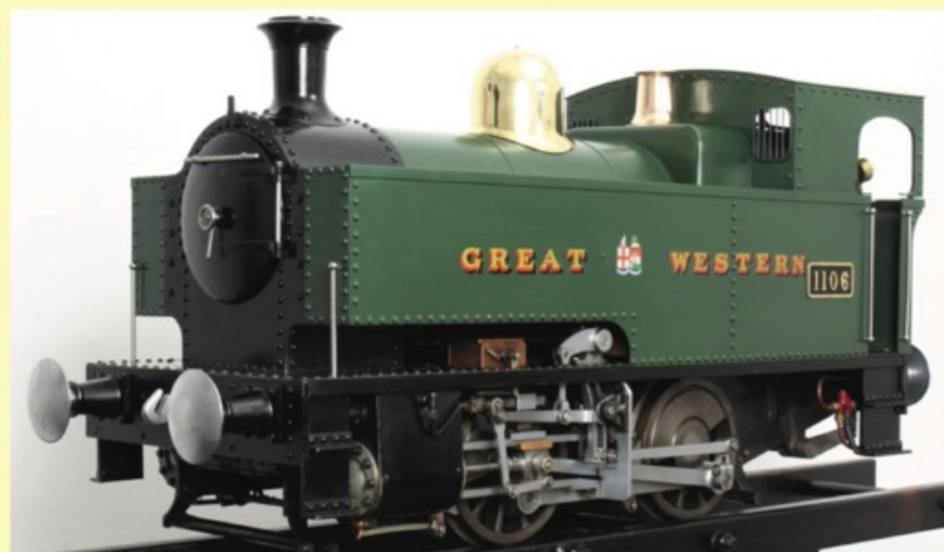
7 1/4 INCH GAUGE GWR 11XX 0-4-0T A well built GWR 11XX dock tank to George Gentry's "Midge" design, published in "Model Engineer" magazine in 1935. It runs well, boiler has had recent test with certification for same. Machining of motionwork and valve gear is very crisp, fit and finish good throughout. £6,750
