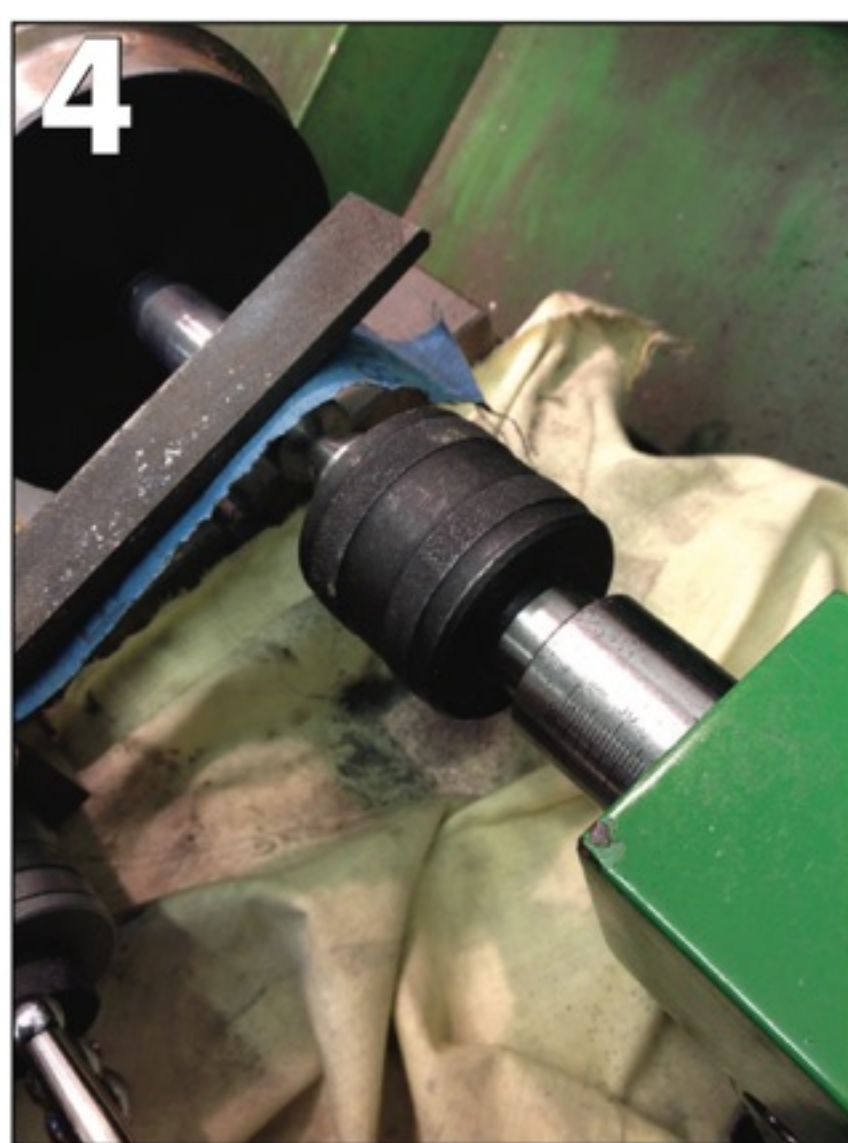
PHOTO 4: Here the axle ends are being polished up with Emery paper to persuade the bearings on.
