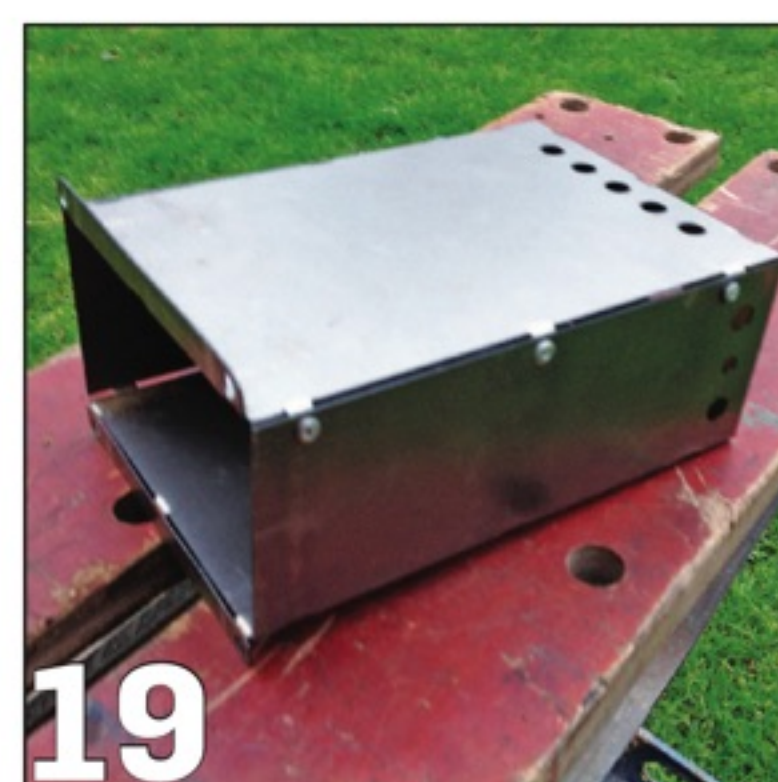
PHOTO 14: First stage in bending up the frame for the bonnet.
