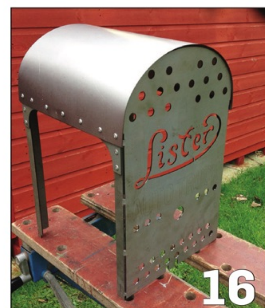
PHOTO 14: First stage in bending up the frame for the bonnet.
