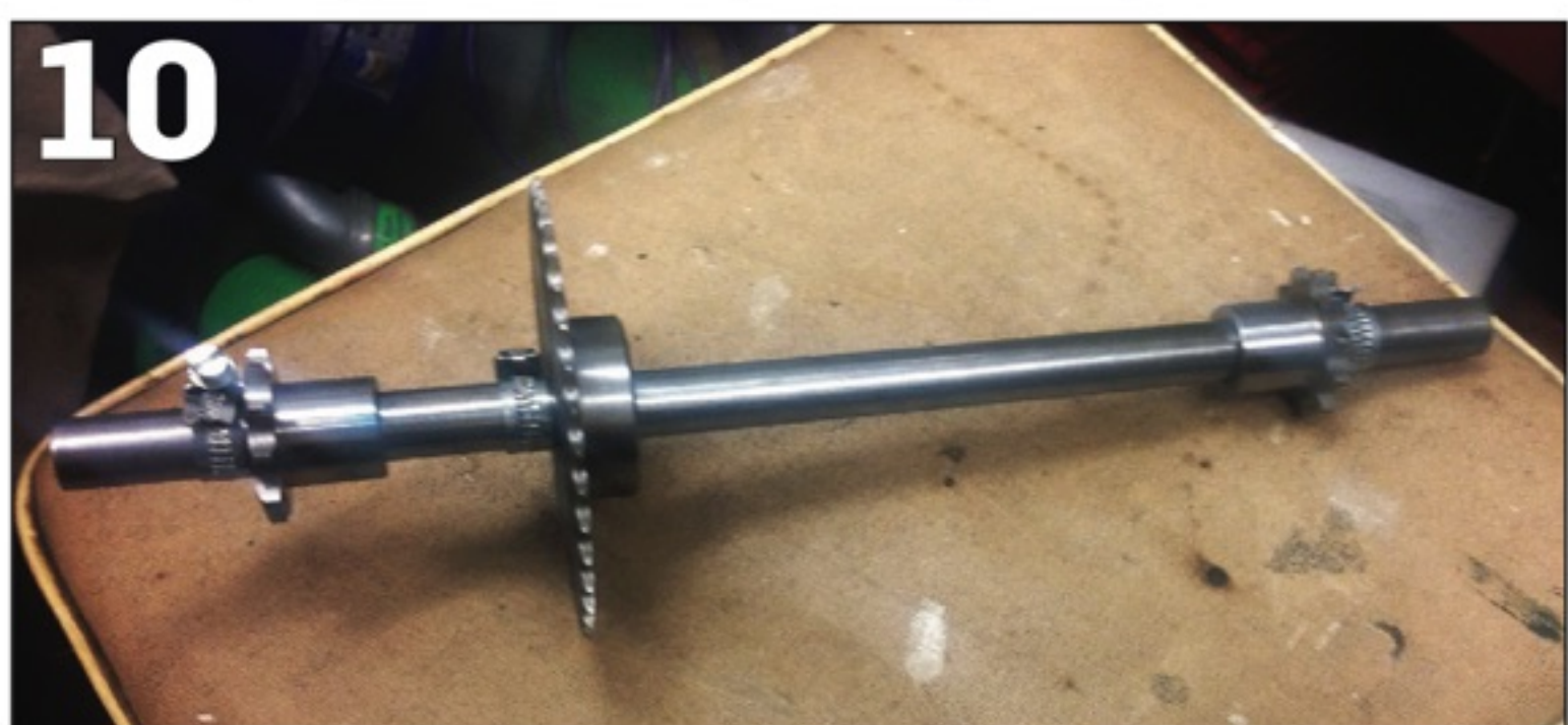
PHOTO 10: Marking-out blue on the layshaft ensures correct positions for sprockets are marked before welding. Jubilee clips hold everything in the correct place temporarily.
