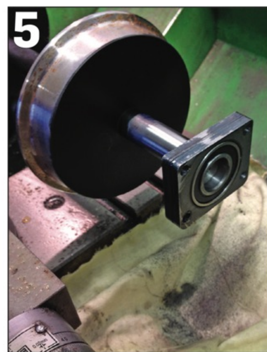
PHOTO 5: Almost there – wheel with its axle almost fitting nice and snugly into the bearing.
