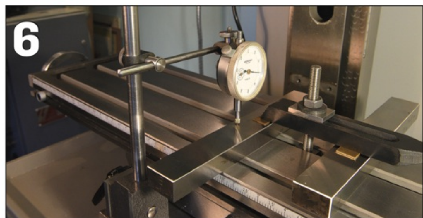
PHOTO 6: ...and the same test for the Y-axis slideway.
