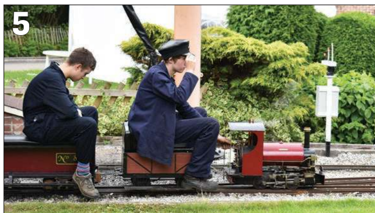
PHOTO 5: Nathan Mills with the Sheffield club's 5-inch gauge 'Hobgoblin' fitted with Joy valve gear.
