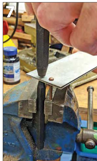
PHOTO 7: Harry using a header and a support to join two plates with rivets. Note the long rivet placed through an adjacent hole to aid accurate lining up of the components.
