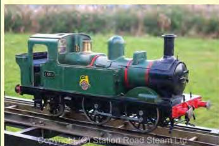
5 INCH GAUGE GWR 14XX We sold this engine a couple of years ago, it's recently come back into stock. A heavily reworked kit engine, it steams and runs well. Paintwork is reasonable, although adorned with rather offensive red boiler bands. The usually rather crude looking motionwork has been bulled up to a decent finish, overall standard of assembly is good. £3,450
