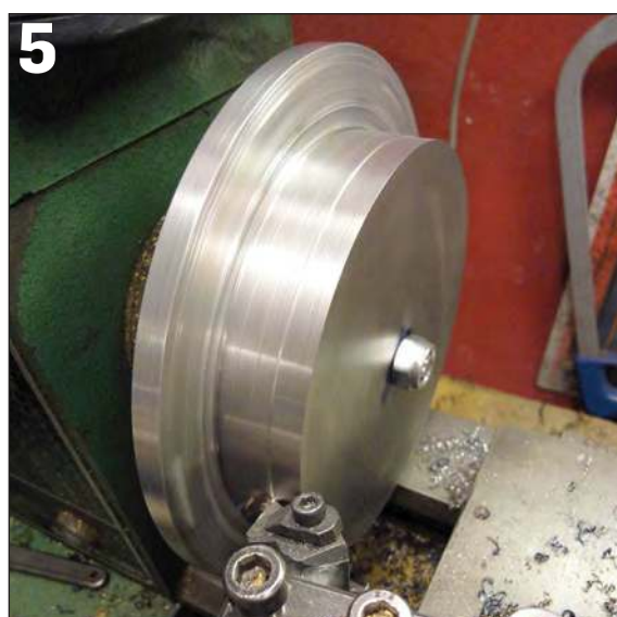
PHOTO 6: Re-centring wheel after flipping it around - this must be done carefully, with high precision.
