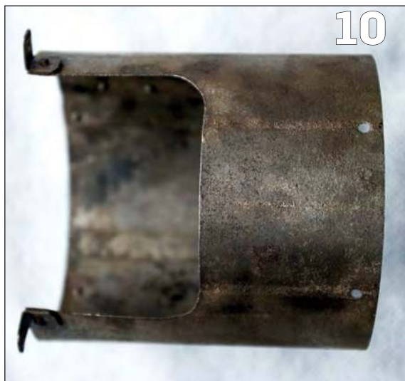
PHOTO 10: The same firebox after the electrolysis de-rusting process had been carried out on it.
