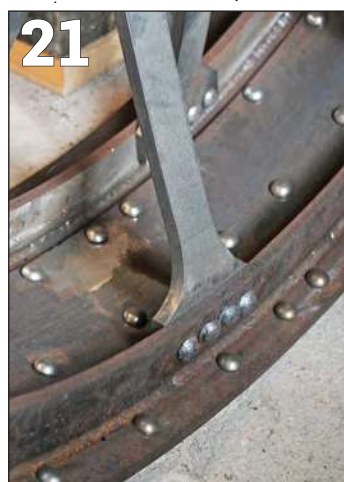
PHOTO 22: Rivet press fabricated from laser-cut components then significantly modified in two planes.
