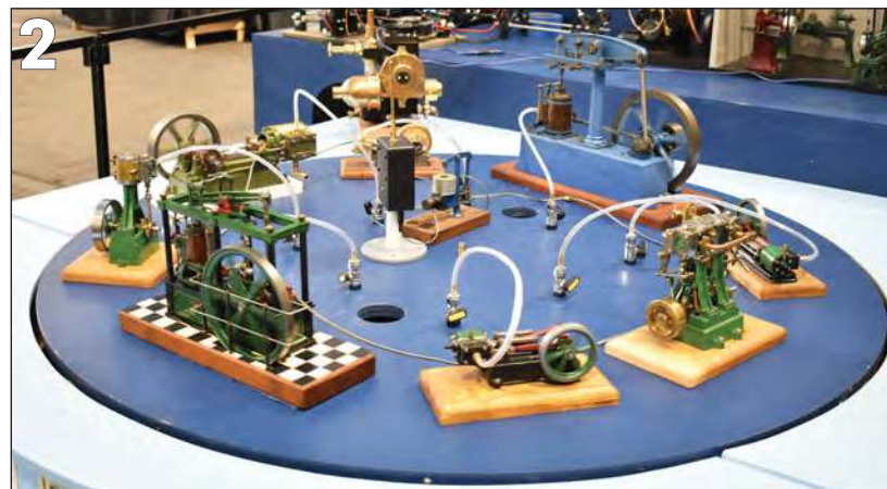
PHOTO 2: The turntable on the Chelmsford stand housed a series of stationary engines, all working on compressed air.
