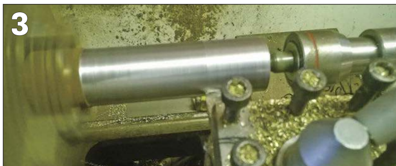
PHOTO 3: Starting point – turning down the mild steel rod.
