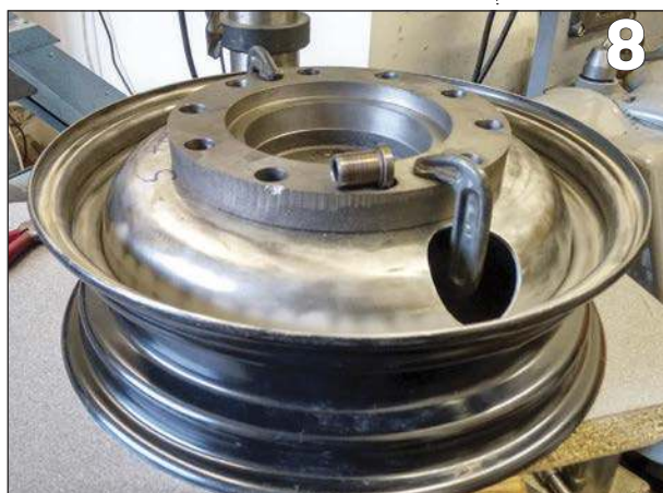
PHOTO 13: Machining a datum face on rear of hub.
