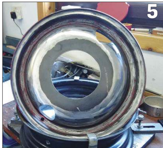
PHOTO 4: Rim carefully clamped for welding in the centre.
