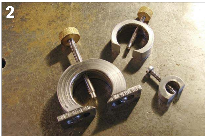
PHOTO 1: Finished puller posed how it would be used on a clock.
