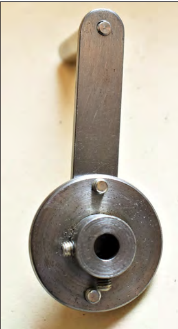
ABOVE LEFT: Completed bearing side plate.
