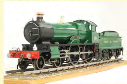
3 1/2 INCH GAUGE "COUNTY OF DORSET" 4-4-0 A new, unsteamed GWR "County" to Don Young's "County Carlow" design. Machining work is crisply executed. Fit and finish of the motionwork is good, the chassis runs well on air. Silver-soldered copper boiler by R Chambers of Weymouth. £3,450
