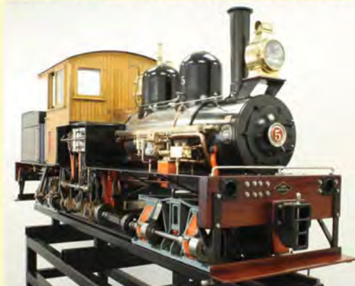
3 1/2 INCH GAUGE GWR PRAIRIE A 3 1/2 inch gauge GWR small Prairie to Martin Evans' "Firefly" design, unsteamed from new. The locomotive has a silver soldered copper boiler by Western Steam with manufacturer's original shell test certificate; needs some work to commission for steaming. £2,650
