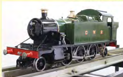
3 1/2 INCH GAUGE GWR PRAIRIE A 3 1/2 inch gauge GWR small Prairie to Martin Evans' "Firefly" design, unsteamed from new. The locomotive has a silver soldered copper boiler by Western Steam with manufacturer's original shell test certificate; needs some work to commission for steaming. £2,650
