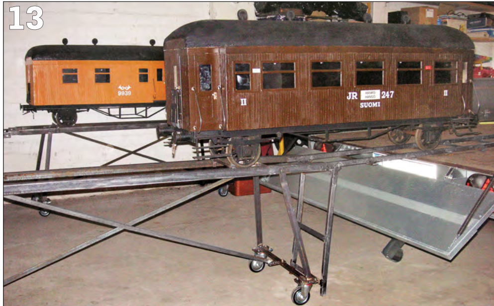
PHOTO 13: Loading rolling stock into a car or onto a trailer is easy and requires no lifting. A simple collapsible ramp spans the distance between the cart and trailer.
