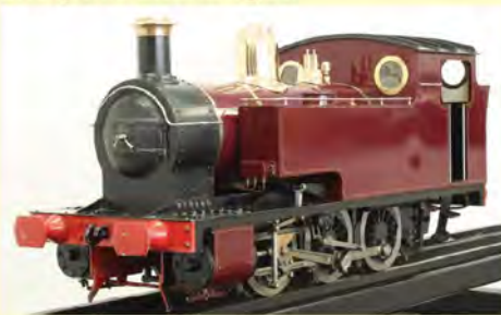
5 INCH GAUGE LMS 0-6-0T "BUTCH" A nicely-built 5 inch gauge 0-6-0T locomotive to Kennions "Butch" design. Machining is all crisply done, fit and finish of the valve gear and motionwork is good. Pretty much ideal as a beginner's engine for either a garden railway or club running. £3,450
