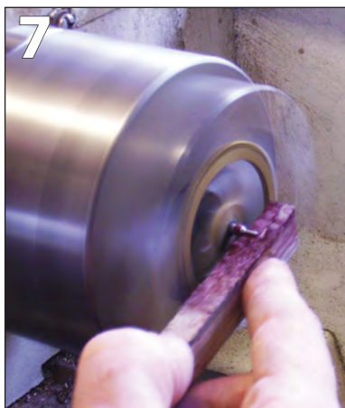
PHOTO 7: A small Dremel felt polishing wheel provides the final touch.
