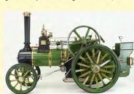
5 INCH GAUGE LMS 0-6-0T "BUTCH" A nicely-built 5 inch gauge 0-6-0T locomotive to Kennions "Butch" design. Machining is all crisply done, fit and finish of the valve gear and motionwork is good. Pretty much ideal as a beginner's engine for either a garden railway or club running. £3,450
