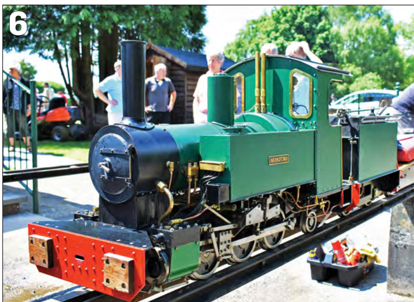
PHOTO 6: Sweet Pea variety 1 – ‘Monjuro’ the 5-inch gauge o-6-2 tender version of the loco fitted with Baker valve gear.
