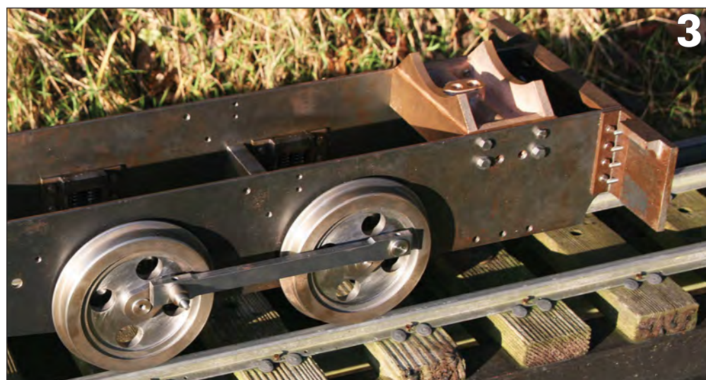
PHOTO 3: Trial fitting of the port and saddle block, checking that all the holes line up correctly.
