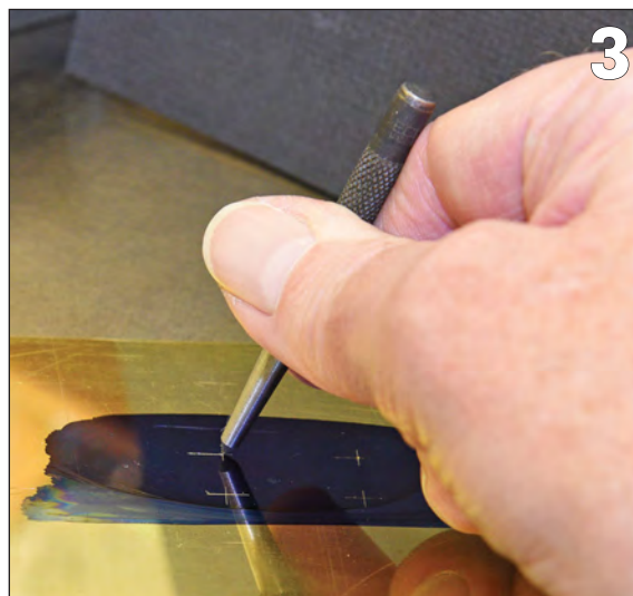
PHOTO 3: Angling centre punch helps with slightly off-target marking.
