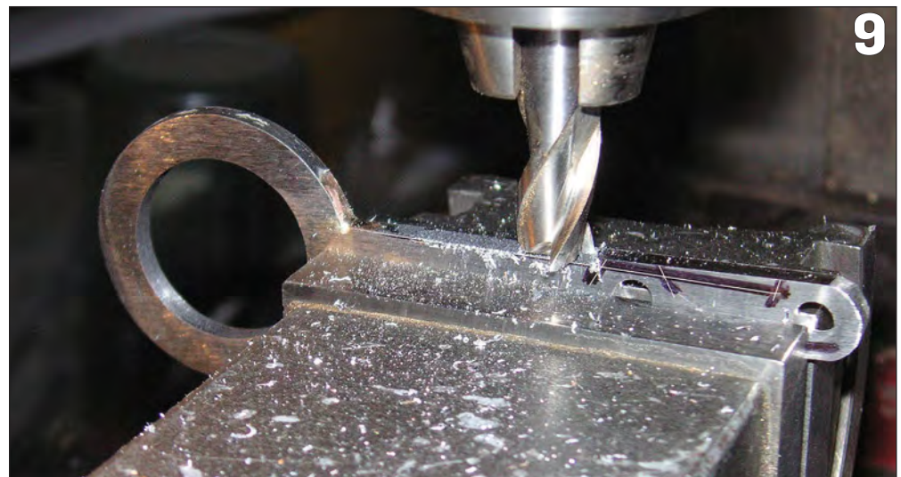
PHOTO 9: Milling outline of eccentric rod to scribed markings.
