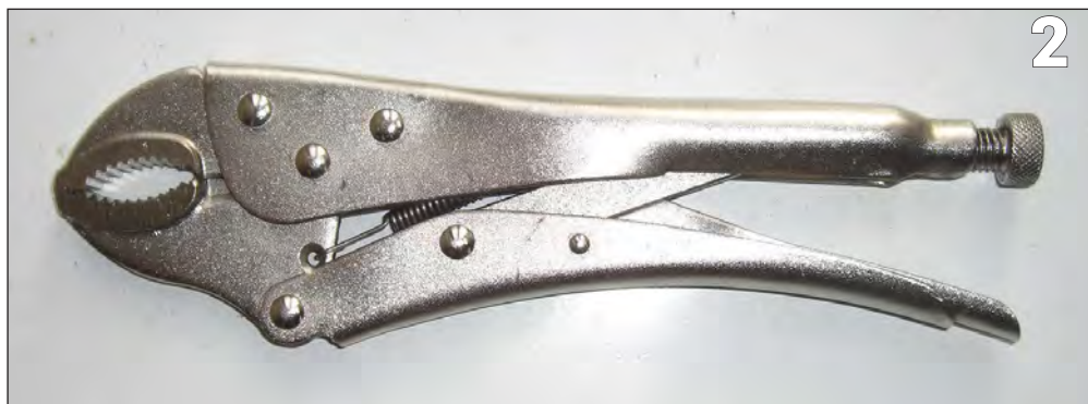
PHOTO 2: Type 1 grips with a riveted fixed jaw used for the conversion.
