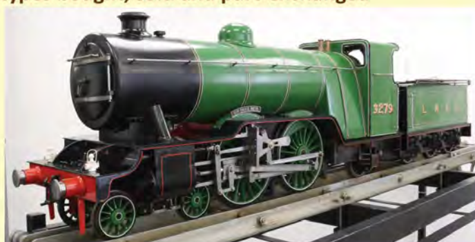
5 INCH GAUGE LNER ATLANTIC 4-4-2 A venerable 5 inch gauge Atlantic, built in 1947 and still in regular club use. Silver soldered copper boiler, 80psi working pressure, feed by twin injectors with hand pump in the tender. Paintwork presentable. £4,950
