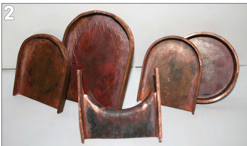
PHOTO 2: Annealed copper plate beaten into shape around formers to produce completed boiler plates.
