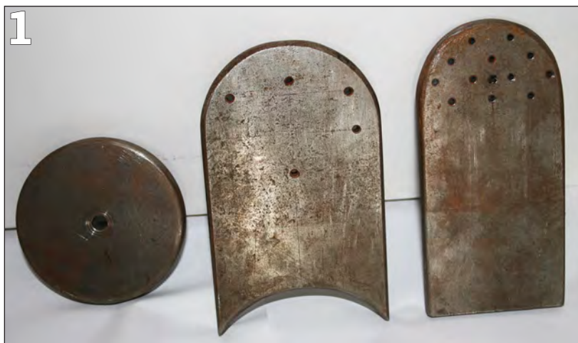
PHOTO 1: Steel formers for firebox, front tubeplate and backhead, edges rounded to avoid denting soft copper.
