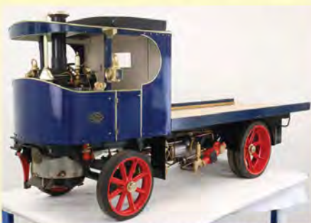
3 INCH SCALE ATKINSON STEAM WAGON A particularly well made 3 inch scale Atkinson steam wagon to the Ray Prime design - it runs beautifully, the engine is very quiet and surprisingly powerful. Commercially-built silver soldered copper boiler by Kingswood, 100psi working pressure. £6,750
