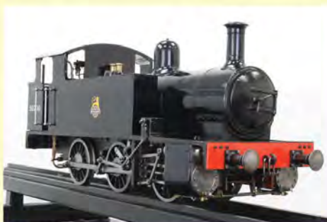
5 INCH GAUGE "SIMPLEX" 0-6-0 A well put together Simplex, it's come to us recently. Silver soldered copper boiler, 100psi working pressure, feed by injector, axle pump and hand pump. Paintwork is presentable, mechanically it runs well. £6,450
