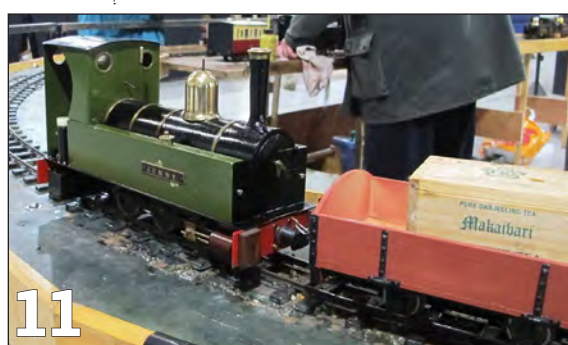
PHOTO 12: Why the steam blower on this 16mm Darjeeling loco? Because it is coal fired – model engineering, just on a smaller scale.
