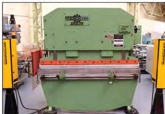
SAGITA BEYELA Type 75-2000: Downstroke Hydraulic Press Brake. Capacity 75Ton x 2000mm. Distance Between Side Frame's 1570mm. Guard Scan Light Guards. £7,950
