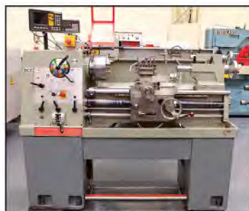
COLCHESTER STUDENT 1800: Gap Bed Centre Lathe. Swing 13". Between Centres 24". Spindle Bore 1 1/4". Speeds 22 - 1800rpm. QCTP. (ex College) £4,950
