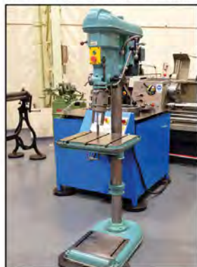
FORCO 10/EIGHT: Pillar Drill. Speeds 51-2650rpm. Table Size 20" x 17". No.3 Morse Taper. Throat 10". £1,850
