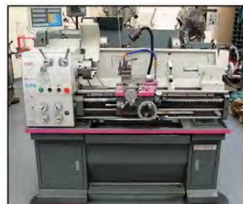
EXCEL Type OPTIMUM D320x920: Gap Bed Centre Lathe. Swing 11". Between Centres 30". Spindle Bore 1 1/2". Speeds 65 - 1800rpm. QCTP. Digital Readout. £2,950
