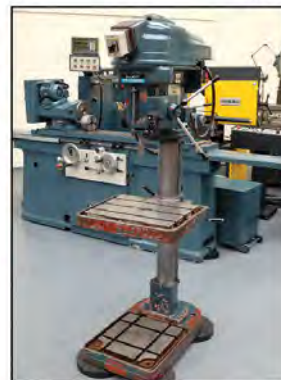
ELLIOTT PROGRESS Type 3A: Pillar Drill. 3 Morse Taper (1" Capacity). Table 19" x 15". Spindle Speeds 110 - 1780rpm. £1,400
