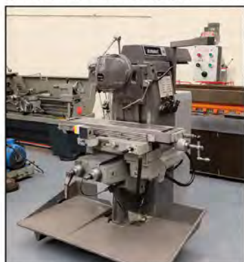
BRIDGEPORT Model 15: Universal Milling Machine. Swivel Vertical Head. Swivel Table Size 42" x 9". Spindle Tapers 40 ISO. Speeds 35 - 1200rpm. £2,750
