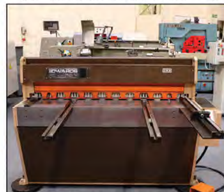
EDWARDS PEARSON Type DD: Power Guillotine. Capacity 1270mm x 2.5mm (50" x 10swg). Manual Back Gauge. Front Supports and Squaring Arm. £5,250
