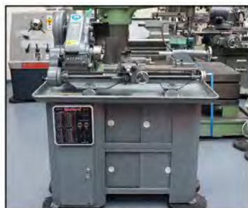
MYFORD SUPER 7: Model Makers Centre Lathe. Swing Over Bed 7". Distance Between Centres 20". Spindle Bore 7/8". 3 & 4 Jaw Chucks. Collet Set. £1,950
