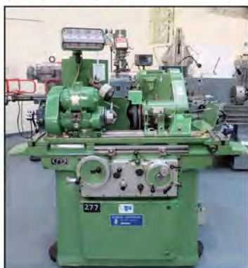
JONES & SHIPMAN Type 1715/39: Cylindrical Grinder. Distance Between Centres 18". Swing Over Bed 8". Swivel Workhead. 2 and 3 Point Steadies. £3,250
