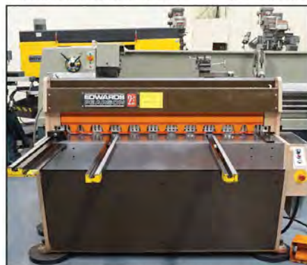
EDWARDS PEARSON Type DD: Power Guillotine. Capacity 1270mm x 2.5mm (50" x 10swg). Manual Back Gauge. Front Supports and Squaring Arm. Ex. University. £5,750
