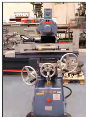
VICTA Type Eagle: Manual Tool Room Surface Grinder. Capacity 10" x 5". Magnetic Chuck. £2,250
