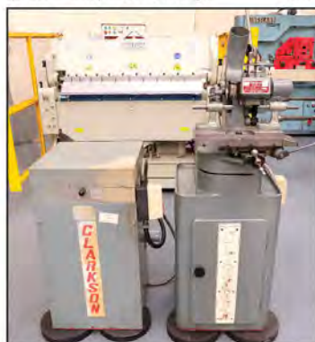
CLARKSON MK2: Tool and Cutter Grinder. Capacity 12" x 6". Pair of Centres. Universal Holder. Dust Extraction. £1,250
