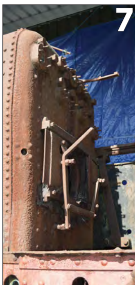
PHOTO 7: Belpaire firebox backhead with all of the non-ferrous fittings missing.
