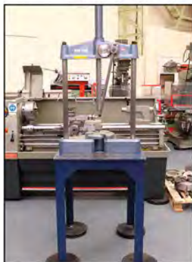
JONES & SHIPMAN: Bench Type Geared Arbor Press. Distance Between Uprights 20". Daylight 24". On Steel Stand. £1,650
