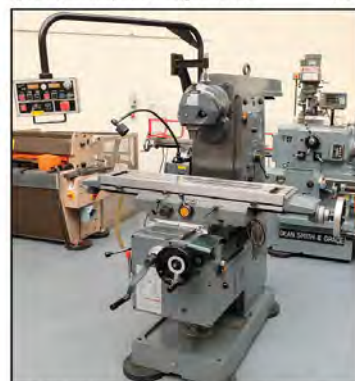
AJAX Model No.1 MK5: Universal Milling Machine. Table Size 43" x 10". Taper 40ISO. Power Feeds All Ways. Variable Speeds 35 - 1800rpm. Pendant Control. £5,250
