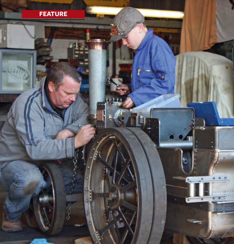
Engine on blocks with hind wheels removed (SAC)
