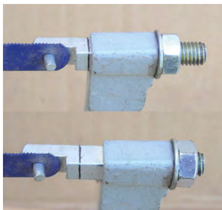
LEFT PHOTOGRAPH 2 Marking the frame to show the correct tension.
