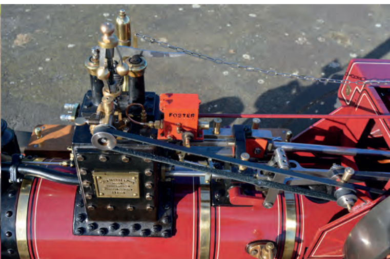
ABOVE: Tom fitted the governor and machined a new pulley wheel.
