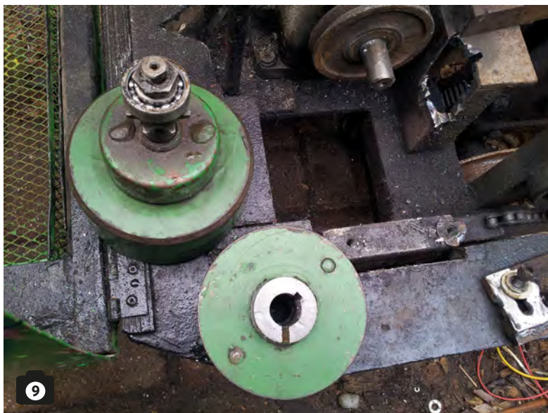
PHOTOGRAPH 9: New clutch assembly showing machined boss and new thrust bearing.
