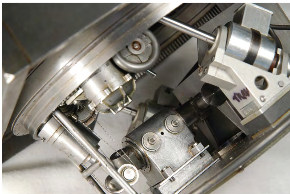
BELOW: Turret platform, uncompleted hydraulic unit, traversing motor.
