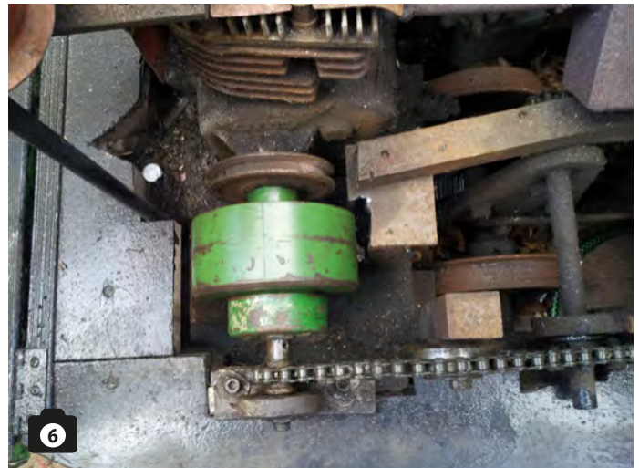
PHOTOGRAPH 8: New clutch showing bigger shoes.
