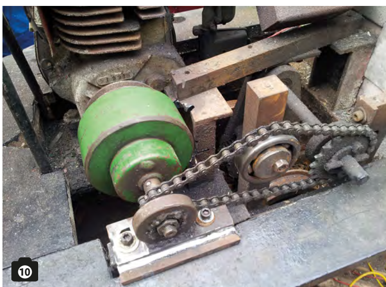
PHOTOGRAPH 10: New clutch in place and ready for action.
