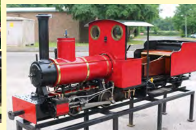
5 INCH GAUGE "ROMULUS" 0-4-0T A nicely built engine, well maintained and steams well. Recently been repainted to a high standard. Steel boiler with expanded tubes, 90psi working pressure, feed by twin injectors. £8750
