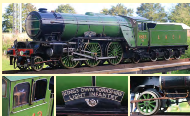
7 1/4 INCH LNER V2 "KING'S OWN YORKSHIRE LIGHT INFANTRY" The work of a highly experienced engineer that was built over twenty years ago. Steel boiler with expanded tubes, 100psi working pressure, feed by injector and axle pump with bypass. Cast iron cylinders with piston valves actuated by Gresley-Holcroft conjugated gear with pole reverser in the cab. Mechanical lubricator. Crank axle is fabricated by press fit and keys, driving wheelsets run in split axle boxes, trailing wheels in prototypical Cartazzi cart. £21500
