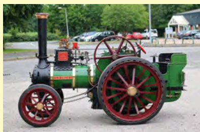
4 1/2 INCH BURRELL AGRICULTURAL A well built engine to the Plastow design. Boiler is sound, it's recently had a twice working pressure hydraulic test and ultrasonic thickness survey. Steel boiler with expanded tubes, 110psi working pressure. £12500
