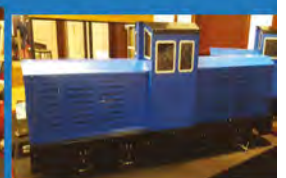
"Imp" £1650 4x motors 4x batteries 100A controller
