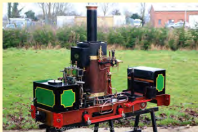
7 1/4 INCH VERTICAL BOILER 0-4-0 A thoroughly well-sorted machine. It runs very quietly, pulls well in both directions and keeps itself in steam and water with minimal attention. Welded steel vertical boiler with expanded tubes, 90psi working pressure. £11500
