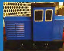
"Pixie" £1350 3x motors 2x batteries 100A controller
