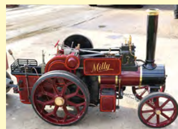
3 INCH SCALE AVELING & PORTER Free-steaming and easy to drive, built in 1996. Copper silver soldered boiler, complete with a matching driving trolley. Free-steaming and easy to drive, Two speed, three shaft transmission, rubber tyres on road wheels. JUST ARRIVED
