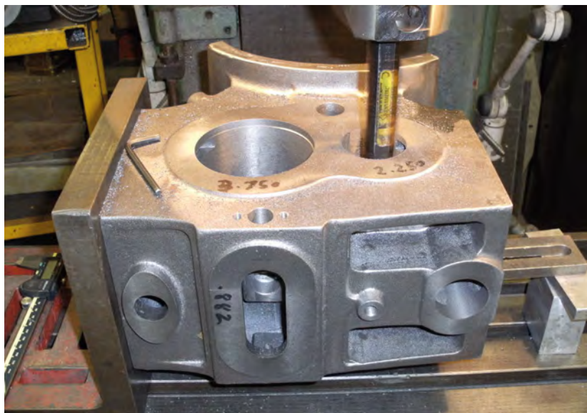
ABOVE LEFT Using a Beaver milling machine to complete the cylinder block.
