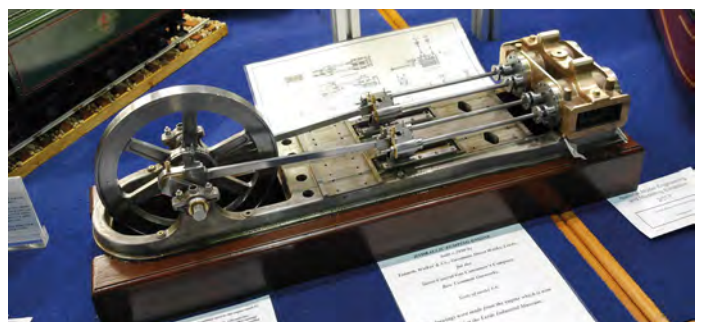
RIGHT – A Tannet Walker pumping engine from the Bradford SME.
