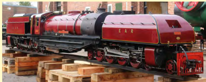
7 1/4 INCH GAUGE EAST AFRICAN RAILWAYS CLASS 59 4-8-2 + 2-8-4 GARRATT A magnificent East African Railways Class 59 Garratt No 5928 "Mount Kilimanjaro", built in 7 1/4 inch gauge by Coleby-Simkins in 1973. Modelled on a metre gauge prototype the model is, predictably, on the large side. Steel boiler with expanded tubes, four element radiant superheater, 150psi working pressure. The engine is fitted for air braking, with steam compressor pump mounted on the smokebox. Length 19' 6" over couplings, weight in running order 2 1/2 tons. £48,500
