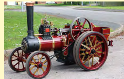
4 INCH SCALE BURRELL AGRICULTURAL ENGINE A new 4 inch scale Burrell, built from a Steam Traction World kit and steamed once. It's been well put together and nicely painted. Welded steel CE-marked boiler, expanded tubes. 120psi working pressure, feed by injector and mechanical pump. Bonded rubber tyres to road wheels. Winch and complete with tender-mounted driver's seat. £16,500
