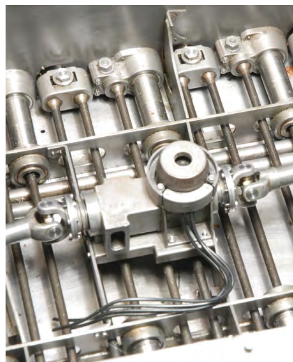
BELOW RIGHT PHOTOGRAPH 37 The power take off unit, situated directly under the turret.
