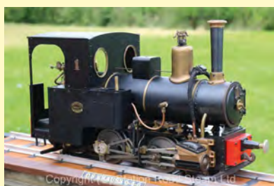
3 1/2 INCH GAUGE OK KRAUSS 0-4-0T Built from an O.S kit twenty years ago and kept for display since, it's in new and unsteamed condition. Silver soldered superheated boiler, feed by axle pump with auxiliary hand pump in the offside side tank. Complete with its original factory assembly instructions and display track. £3,250
