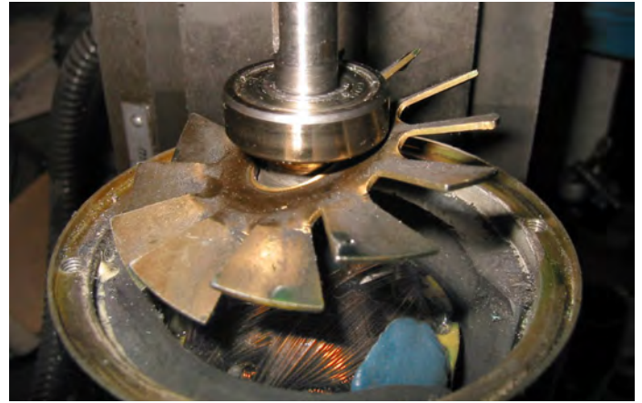
LEFT – PHOTOGRAPH 5 – A close-up of the cutting of the keyway.
