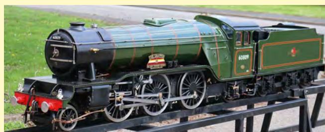
7 1/4 INCH GAUGE LNER V2 2-6-0 "THE SNAPPER" A well engineered 7 1/4 inch gauge LNER V2, in super condition, mechanically it runs very well, fit and finish of the valve gear and motionwork is good, the engine is nicely detailed throughout. Both engine and tender are vacuum braked. Silver soldered copper boiler by Swindon Boilers, 100psi working pressure. Four element radiant superheaters, feed by twin injectors. Twin pop type safety valves. Cast iron cylinders with piston valves actuated by Gresley-Holcroft conjugated gear £26,500
