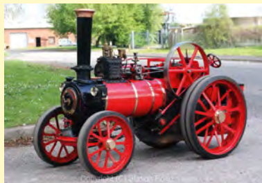
4 INCH FOSTER TRACTION ENGINE Steel boiler, re-tubed three years ago. It steams freely and runs very well. Welded steel boiler with expanded tubes, 120psi working pressure, feed by injector and mechanical pump. Complete with a tender-mounted driver's seat with footrests. £14,500
