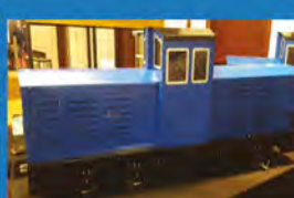
"Imp" £1650 4x motors 4x batteries 100A controller
