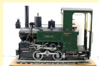
5 INCH GAUGE ORENSTEIN & KOPPEL 0-4-0 Unsteamed from new, the silver soldered copper boiler has had a twice working pressure hydraulic test and the engine has been run on air. Complete with display track. £5,950
