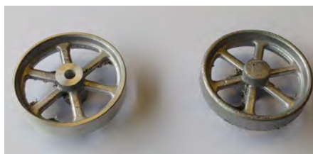
BELOW The wheels before and after machining the outside rim.
