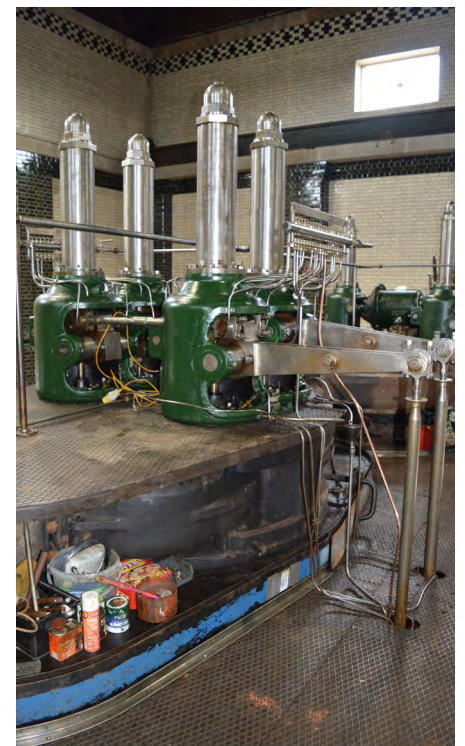
BELOW The upper part of the medium pressure cylinder of Engine No. 7 is shown in this illustration. Note that by way of contrast with the preceding view, owing to the larger size of the cylinder, two inlet and two outlet valves are necessary at each end. The respective sets of valves (inlet and outlet) are worked by a single rocker arm and coupled together by a rod as can clearly be seen here.
