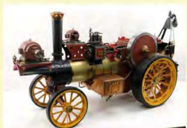
2 INCH SCALE BURRELL DCC SHOWMANS An exceptionally well built Burrell Showmans engine, built to Ronald H Clarke's highly detailed "Thetford Town" design, around 80% complete. The motionwork is silky smooth to turn over, fit and finish of machined parts excellent. £10,500
