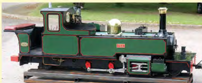
7 1/4 INCH GAUGE LYNTON & BARNSTAPLE 2-6-2T "YEO" In excellent mechanical order throughout, paintwork is in good order - a fine model of a most attractive prototype, built by Milner Engineering. Weighing in at over a ton, it's a powerful engine. Welded steel CE-marked boiler with expanded tubes by Bell Boilers, fitted new in 2014. 120psi working pressure. The engine is fitted with a powerful steam brake, with commercial spec actuating valve in the cab. Whistle is from a Circle Line C69 train. £21,500
