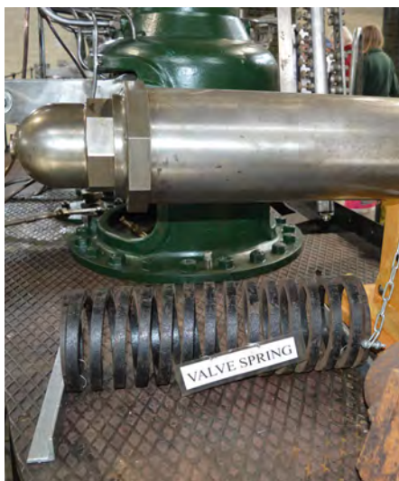
BELOW – One of the valve springs, removed from its accompanying casing, for the high pressure cylinder of Engine No. 7 is shown in this view.
