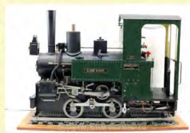
5 INCH GAUGE ORENSTEIN & KOPPEL 0-4-0 Unsteamed from new, the silver soldered copper boiler has had a twice working pressure hydraulic test and the engine has been run on air. Complete with display track. £5,950
