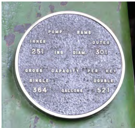
ABOVE – This plaque on Engine No. 6 denotes the pump ram capacity in single and double ram modes of operation.
