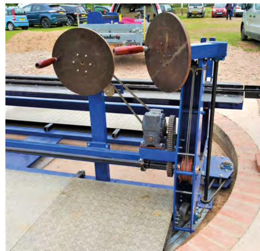
ABOVE A closer view of the operating handles and the rotating and lifting machinery.
