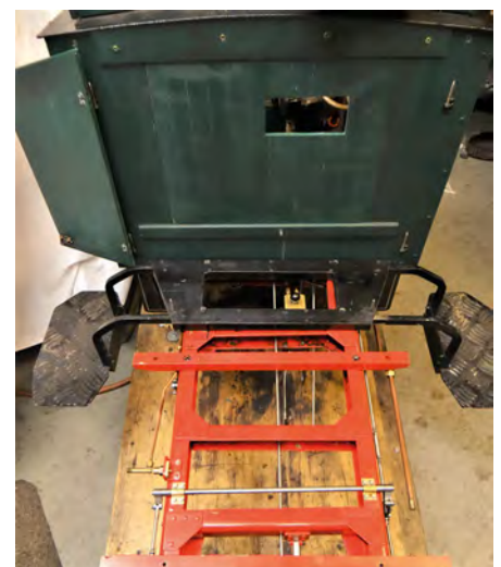
BELOW – PHOTOGRAPH 8 Foot rest plate, tank mounting and side sheets.
