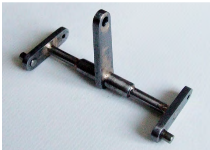
LEFT – PHOTOGRAPH 2 The fabricated brakeshaft assembly cleaned up and ready to fit between the pivot bosses.
