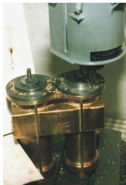
RIGHT PHOTOGRAPH 2 Drilling the cylinder mounting holes.
