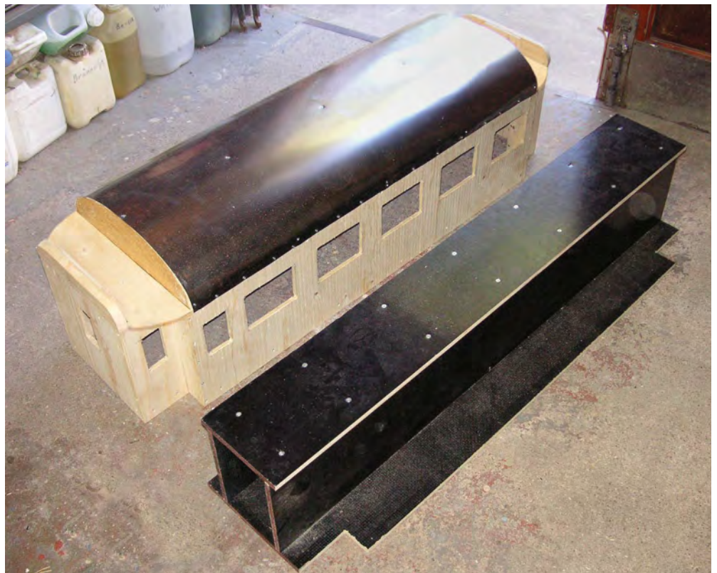
BELOW PHOTOGRAPH 12 The roofing is in place. Note the round-edged plywood ceiling piece over the vestibule.
