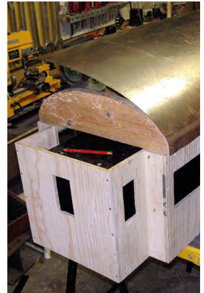
LEFT PHOTOGRAPH 10 Bending the edge of the thin sheet metal to shape.
