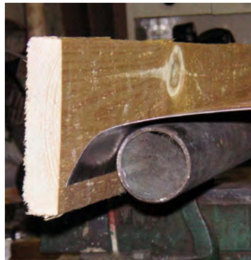
LEFT PHOTOGRAPH 10 Bending the edge of the thin sheet metal to shape.
