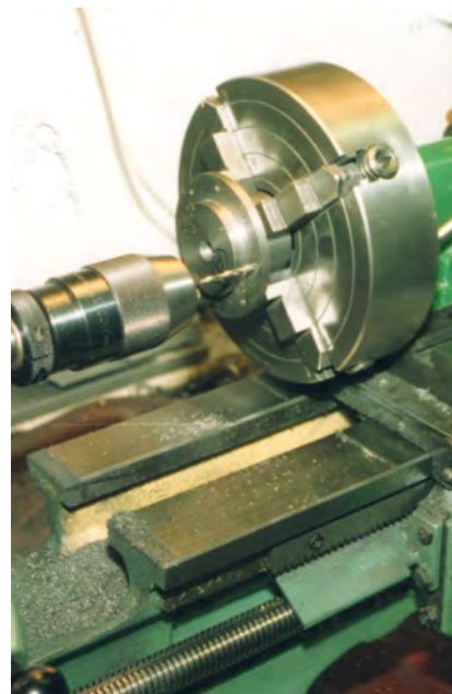
RIGHT PHOTOGRAPH 1 Drilling the rear cover mounting holes.
