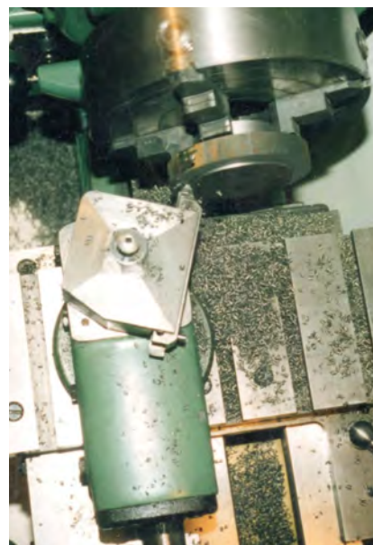
RIGHT PHOTOGRAPH 3 Roughing out the front cover.
