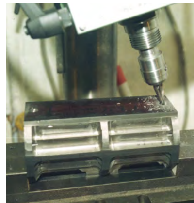
LEFT PHOTOGRAPH 5 Cutting the long steam way.
