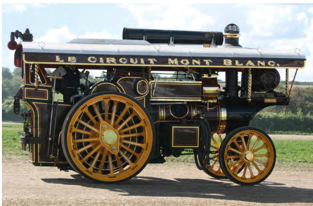
BELOW RIGHT PHOTOGRAPH 10 'Onward', a full-size replica built from original Fowler works drawings and completed this year.
