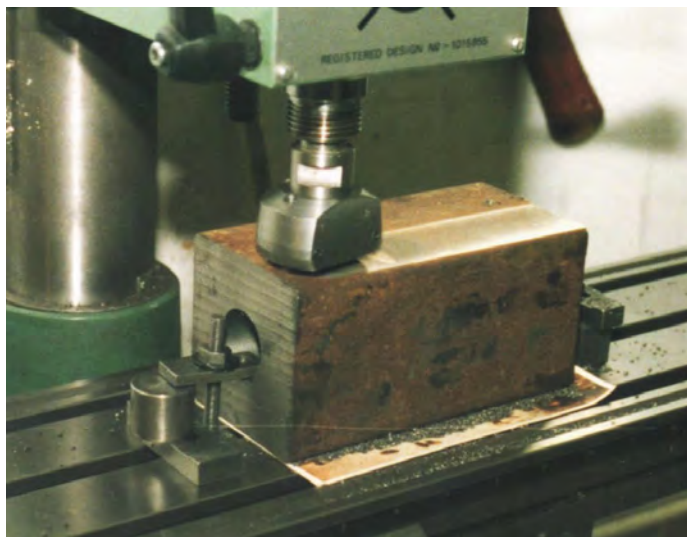
ABOVE LEFT PHOTOGRAPH 1 The initial fly-cut of the cylinder block.
