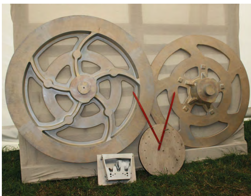
RIGHT PHOTOGRAPH 8 The pattern for the final drive gear wheel on 1908. The pattern is in two halves and the core box used to make all the individual cores for the gear teeth is laid on the grass below. The item like a clock was a device to double check the alignment of all the gear teeth cores to ensure an even spacing of the cast teeth.
