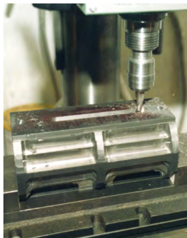
LEFT PHOTOGRAPH 5 Cutting the long steam way.
