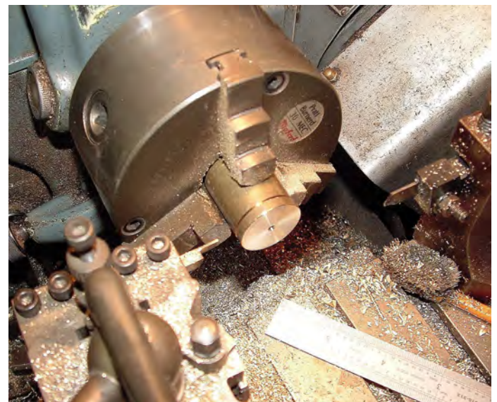
Parting off the regulator disc valve from a 1" brass bar.
