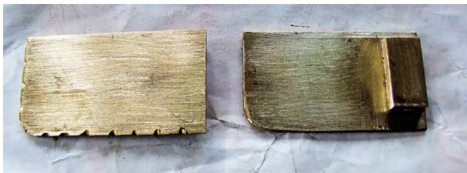
Photograph 10 – The two infill plates fitted in front of the cab structure, notched to fit inside the side sheet fixing angle rivets and with the addition of the thickening plates for the fastenings.
