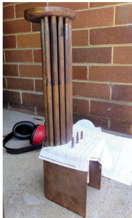
The boiler begins to take shape.
