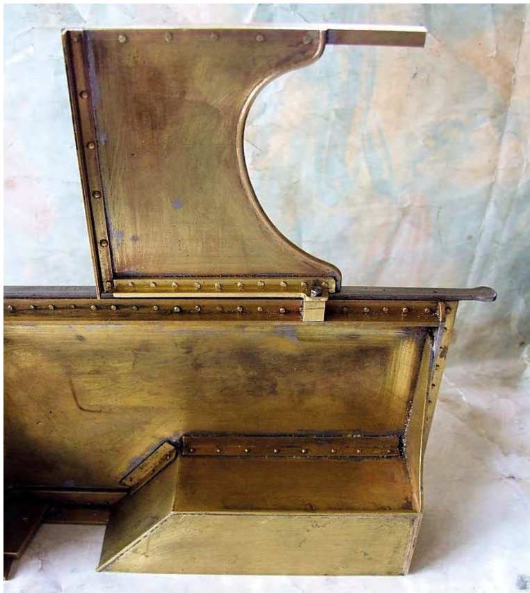
Photograph 2 – The formed roof plate and the profiled cab front shown fitting well together.
