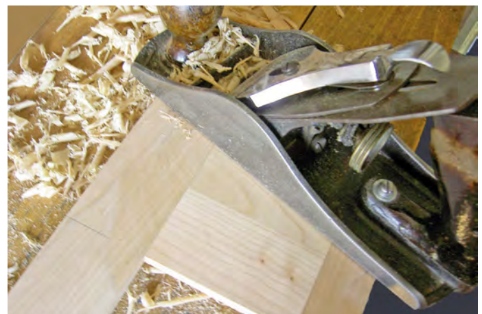
Photograph 57 – Cleaning up a side frame.
