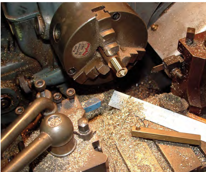
Making the front boss for the regulator. You can just see here that I have put a generous countersink in the end to assist when fitting the main steam pipe as you will have to do this more by feel than sight.
