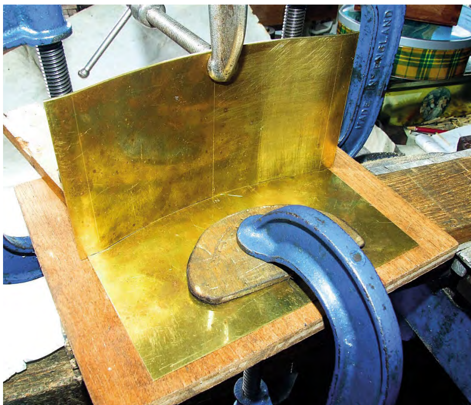
Photograph 2 – The formed roof plate and the profiled cab front shown fitting well together.
