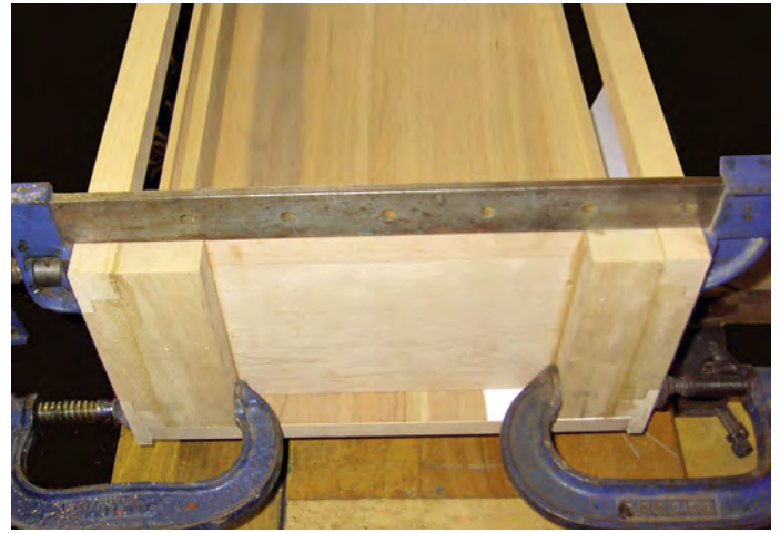
Photograph 59 – Fitting the top panel.
