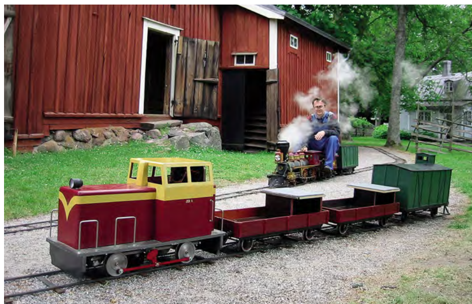
Photograph 1 – 'Quickie' waits for passengers while the author demonstrates his 4-4-0 live steamer at a museum in Ekenäs, Finland. Five hundred feet of portable track was laid on the gravel walks.
