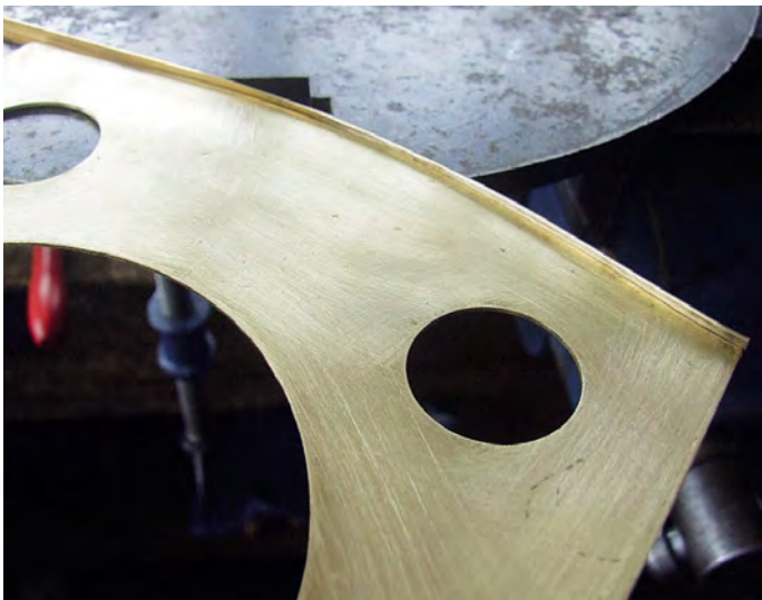
Photograph 8 – Checking the curvature of the angle against the top of the cab front plate.
