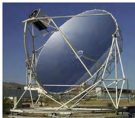
Using solar energy: Solo Stirling engine on solar concentrator.
