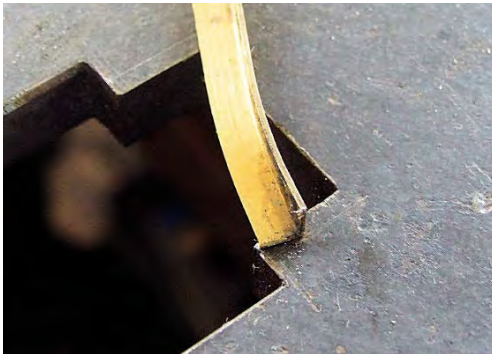
Photograph 8 – Checking the curvature of the angle against the top of the cab front plate.
