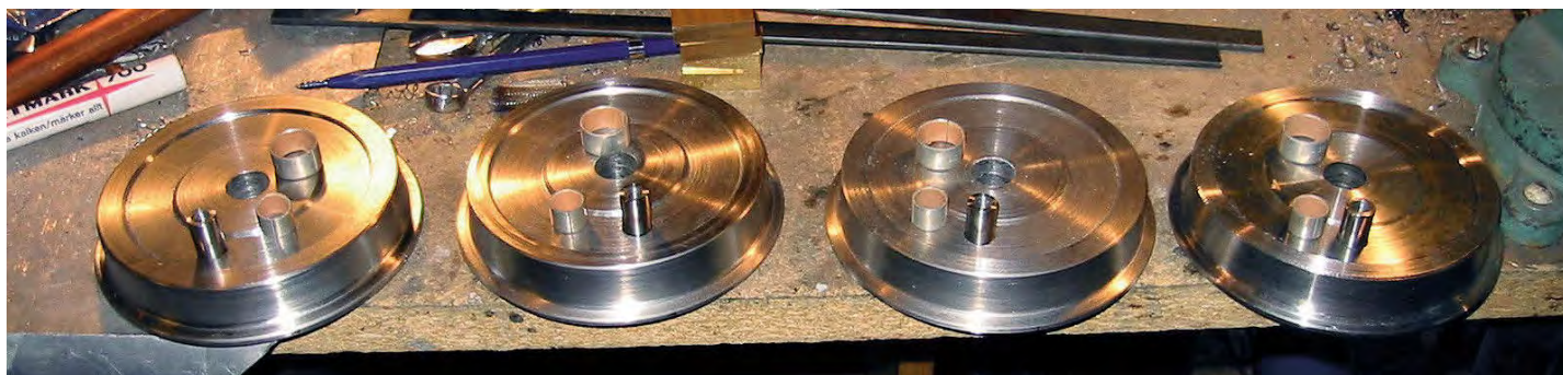
Photograph 2 – Wheels turned from slices of bar stock. The crankpins are already fitted to the wheels. PTFE-coated sleeve bearings are also shown.
