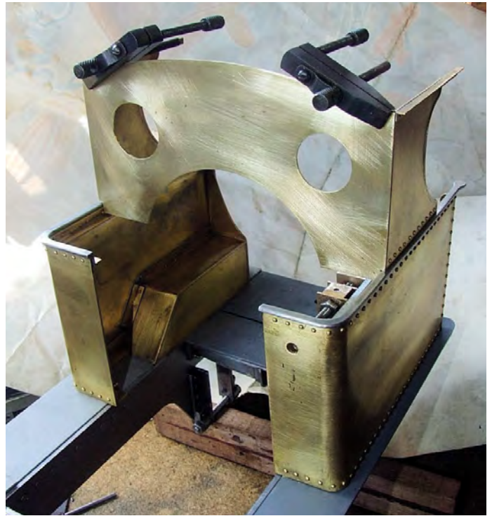
Photograph 6 – Checking the size of the cab front against the assembled side panels.
