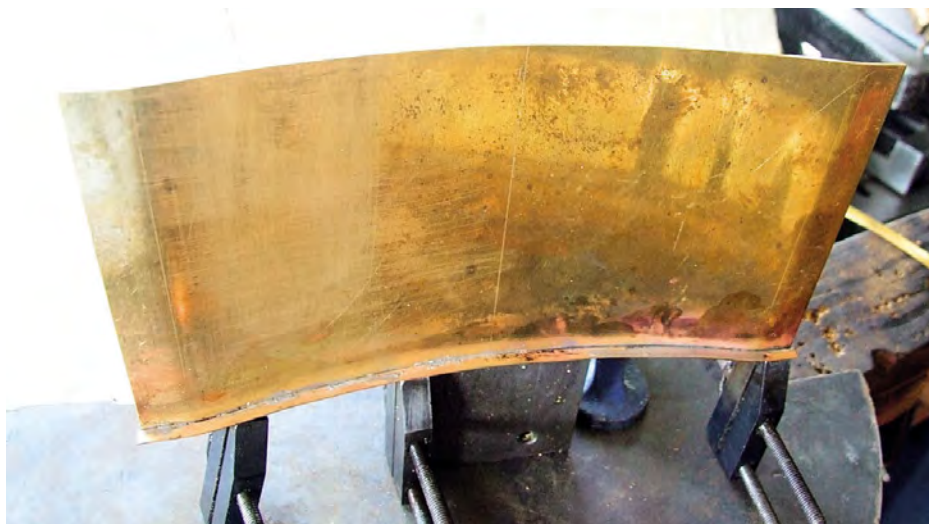
Photograph 12 – Carrying out a similar operation to attach the upper angle with small blocks to ensure the pressure goes on the contact flange and not the edge.
