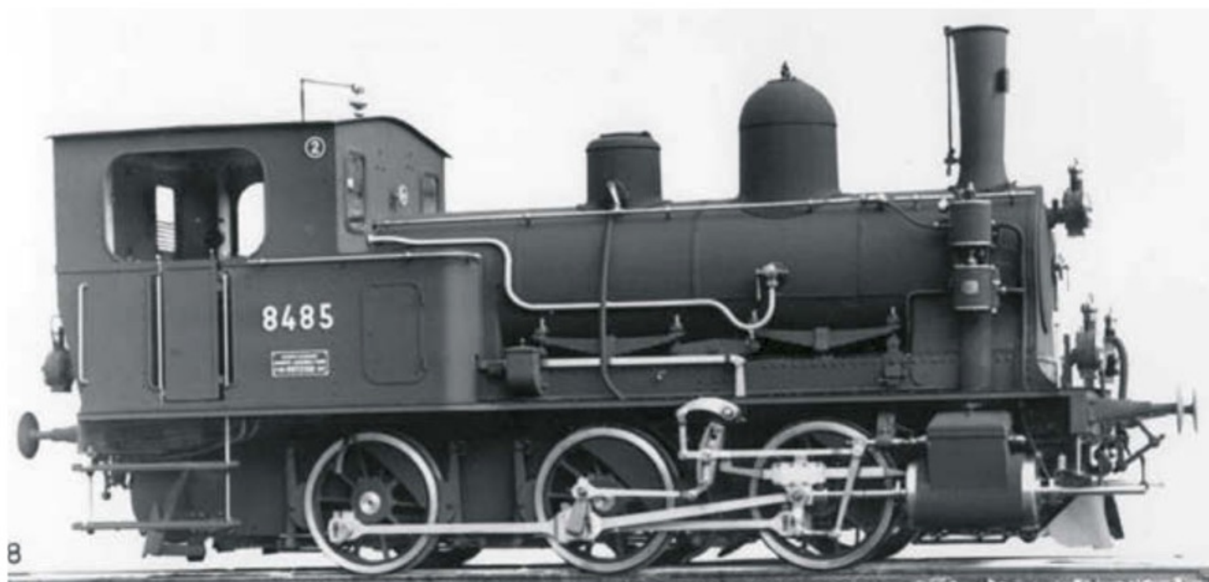
SLM works view of short version E 3/3 'Tigerli' in 1908. Later modified with front platform. Photograph: SLM
