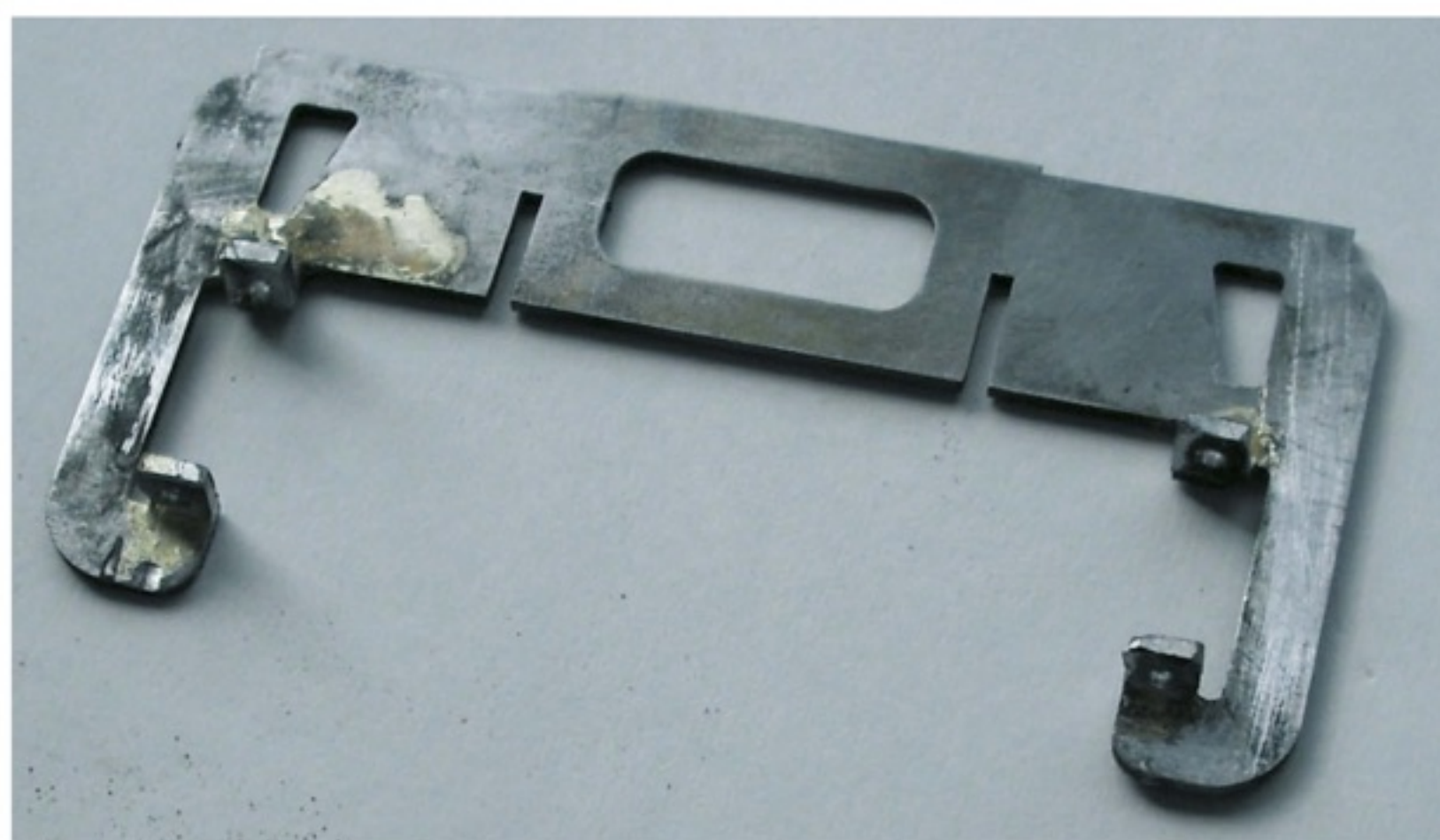
Right: Motion bracket with lugs added for slide bars.
