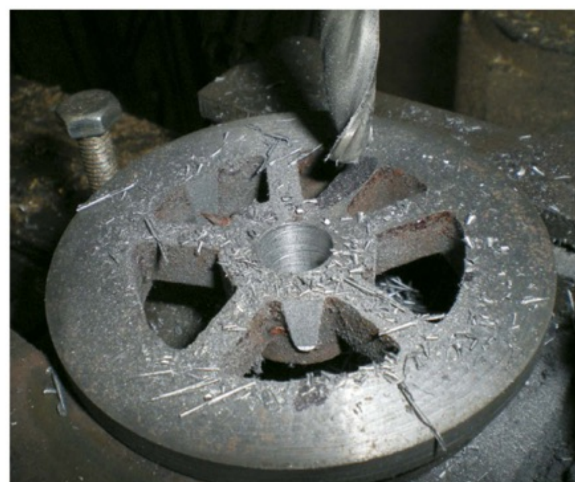
Milling away the extra spokes to produce a more realistic wheel.
