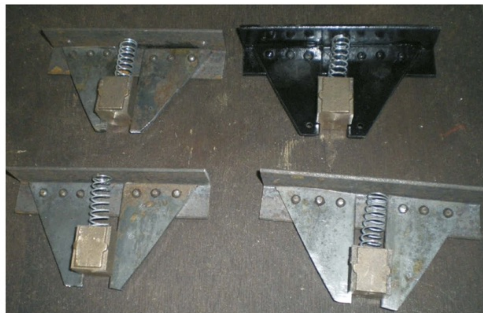
Fabricated axle horn plate parts.
