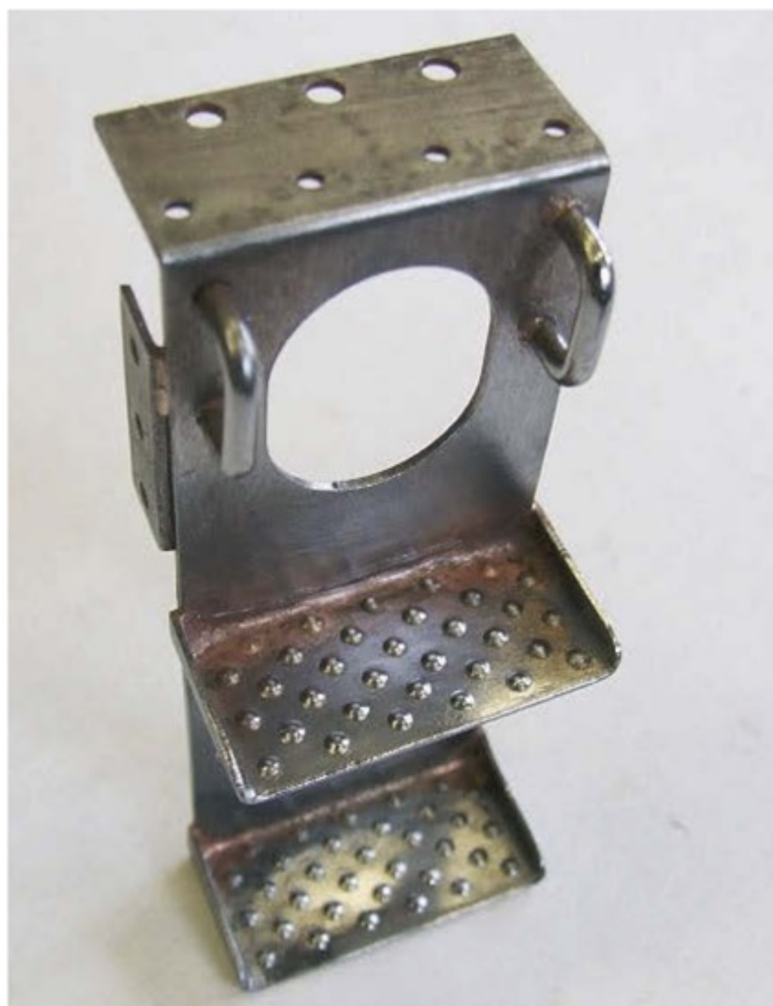
Below: A completed front step.
