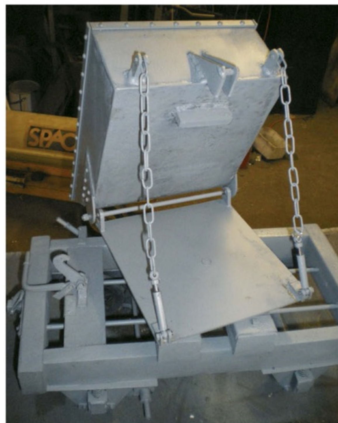
Left: Details of the spring dampers fitted to the skip chains.
