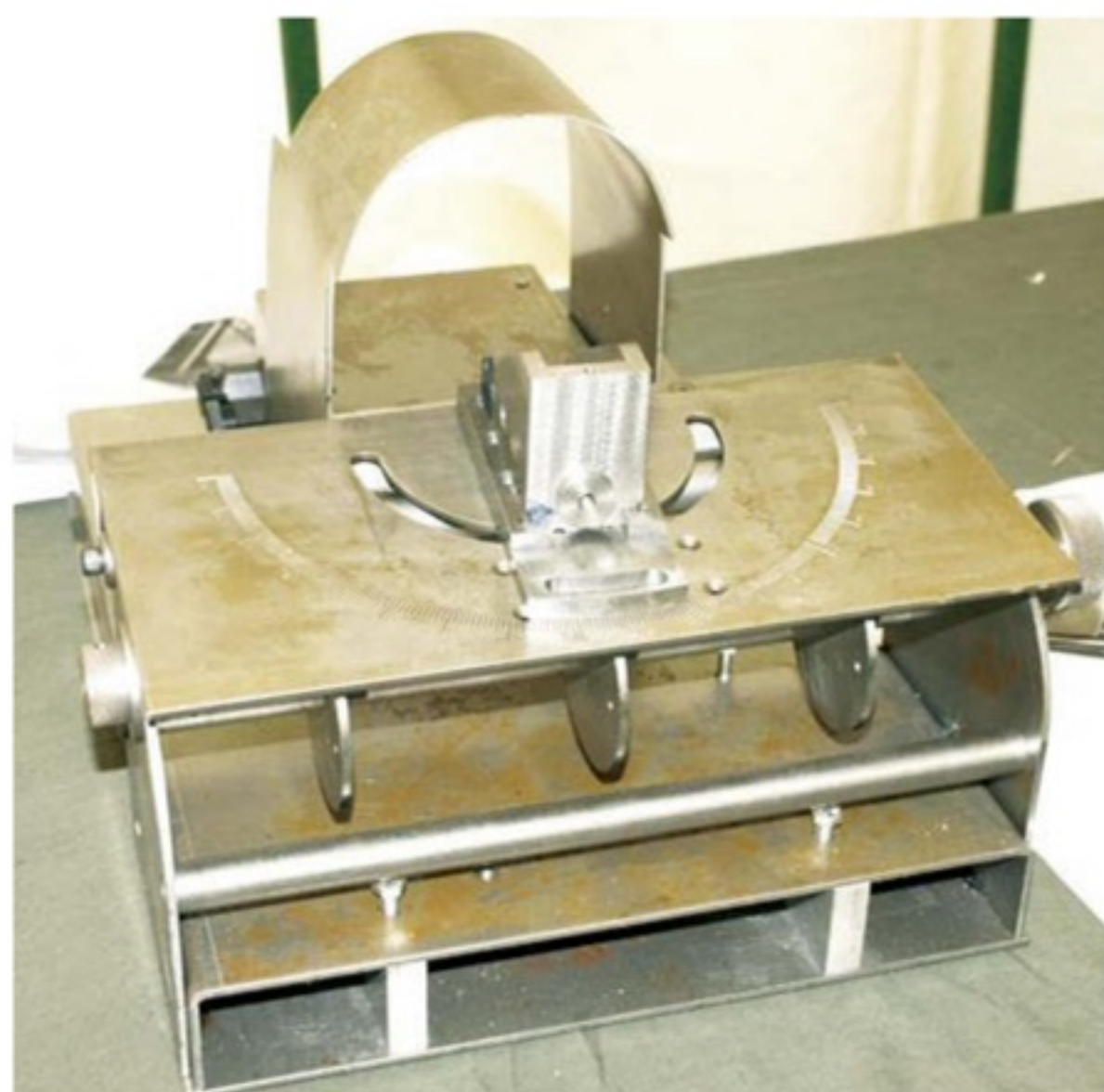
Above: The 'Worden' Mk 3 Cutter Grinder under construction by Nigel Linwood.
