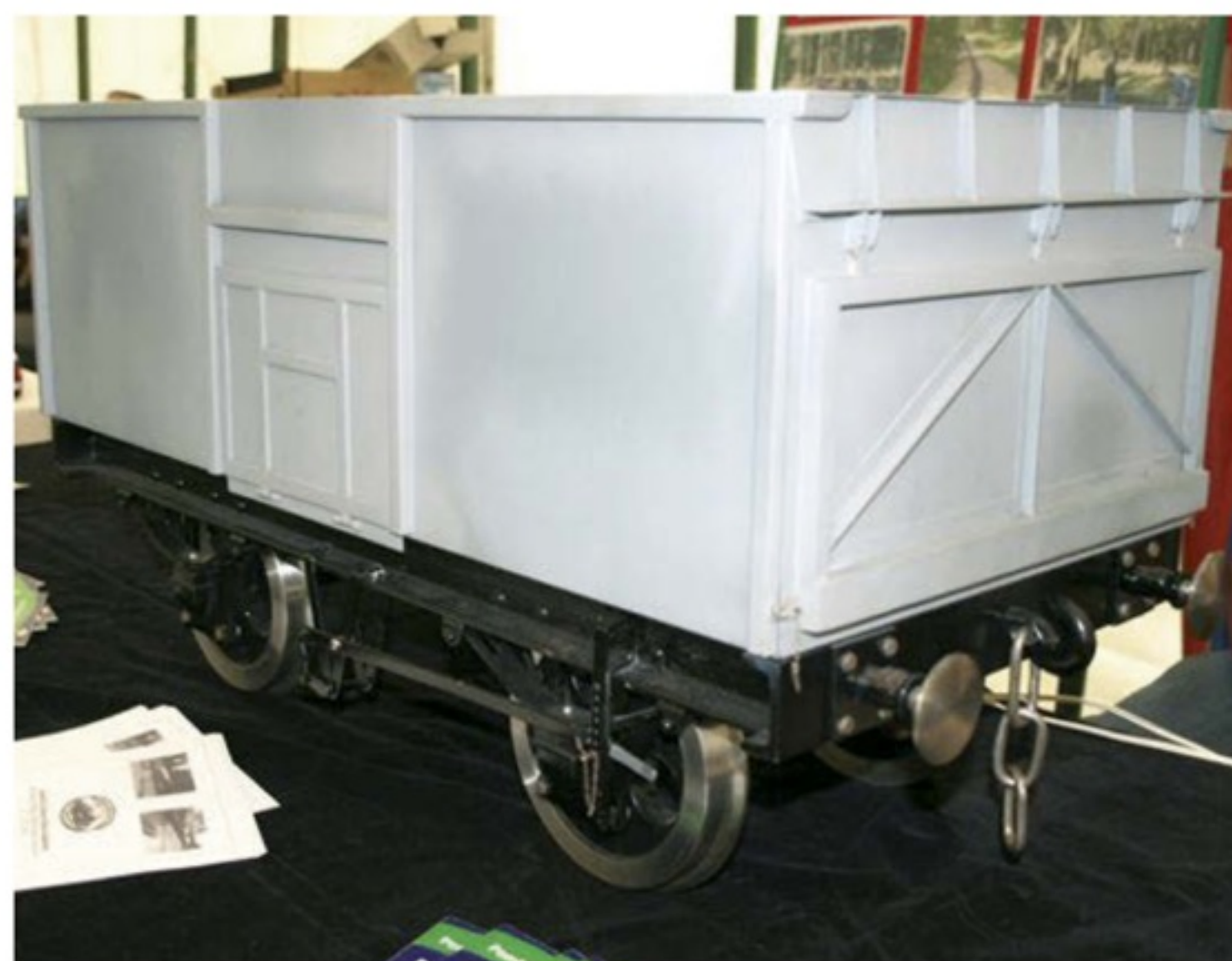
Above: A fine 7 1/4" gauge scratch built 16ton Coal Wagon built by Garth Mosey.
