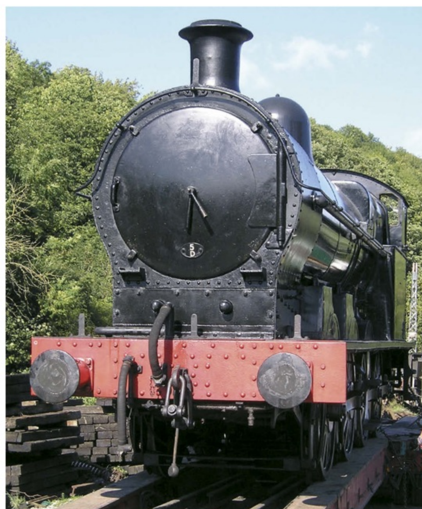
Two views of the preserved G2A Class locomotive on the North Yorkshire Moors railway showing the smoke box detail including the boiler valve and handrail arrangement.
