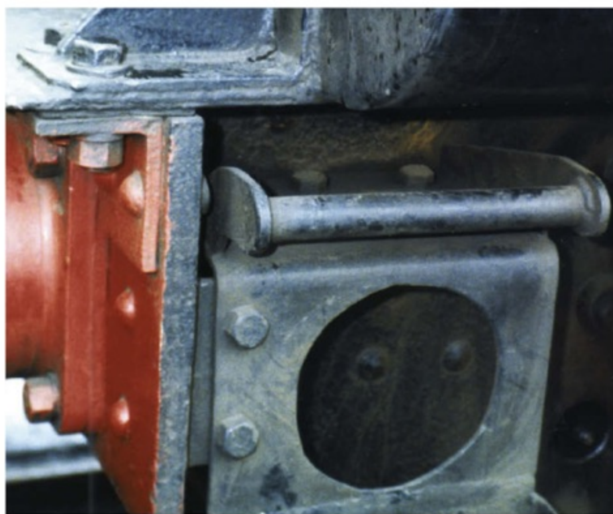
Left: Detail of the handrail on the RH rear of the BR1F tender at Loughborough (Photograph courtesy of Pete Lang).
