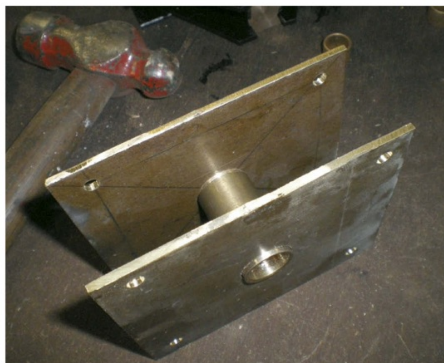
Machining the plates for the pivot tube on which the tipping body rotates.
