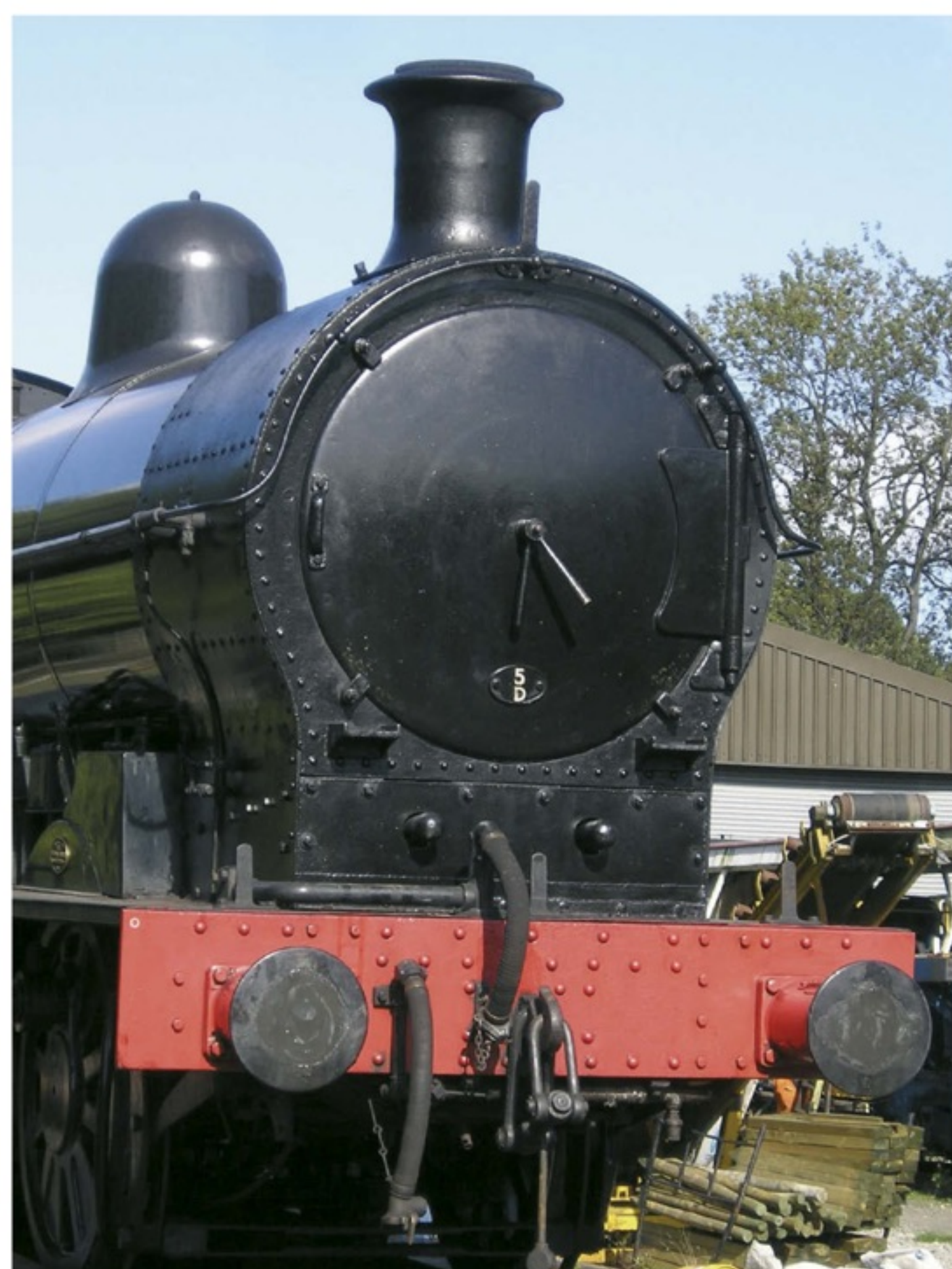
Two views of the preserved G2A Class locomotive on the North Yorkshire Moors railway showing the smoke box detail including the boiler valve and handrail arrangement.
