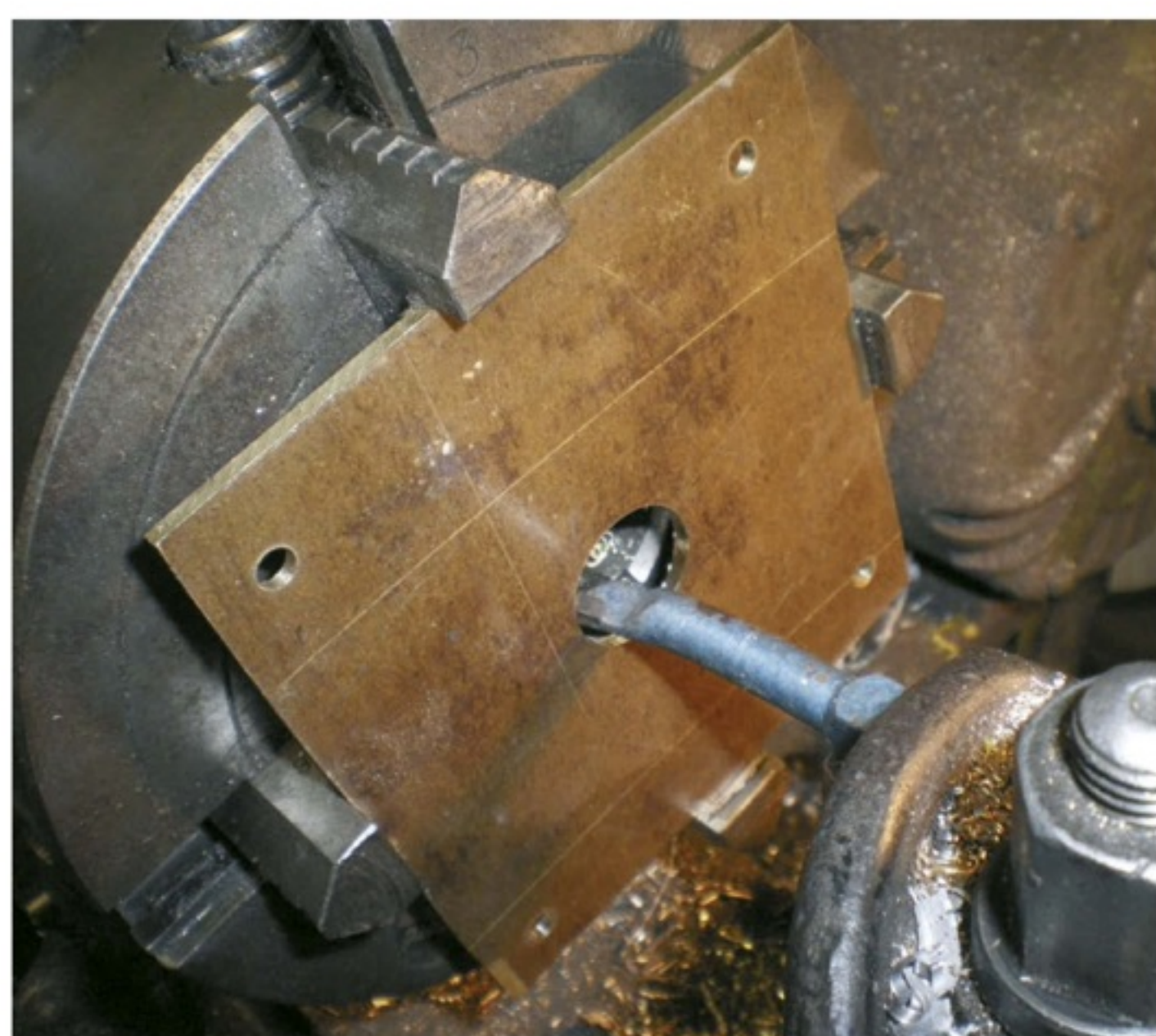
Machining the plates for the pivot tube on which the tipping body rotates.
