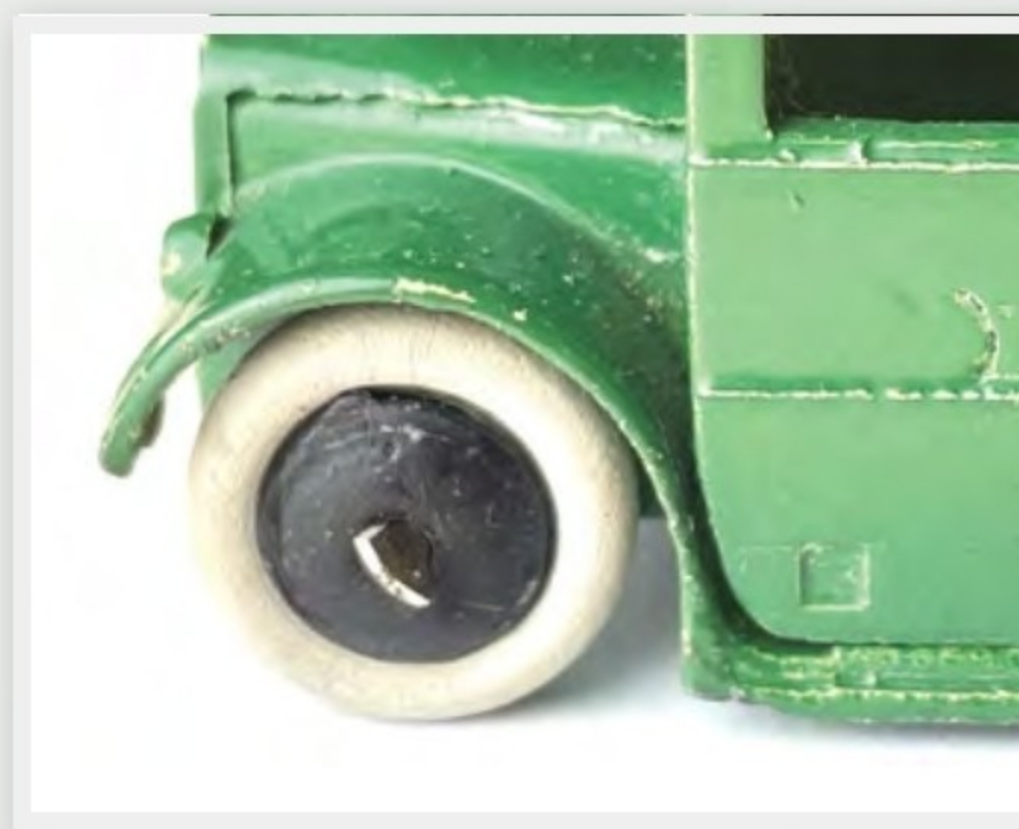
ABOVE A Dinky toy bus displays the nipped axle ends typical of many pre- and post-war models.
