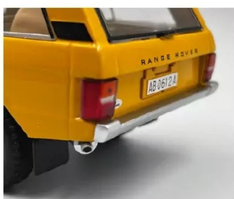
ABOVE This yellow Whitebox shows the correct single tailpipe exhaust fitted to the early Range Rovers.
