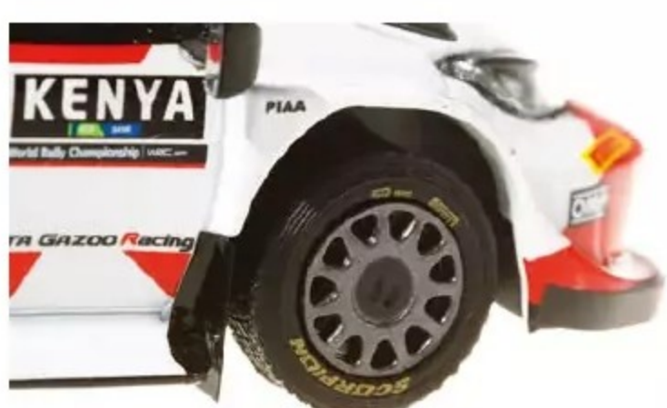
ABOVE Narrow and relatively small wheel rims are necessary for the rough roads that had to be tackled by modern WRC cars.
