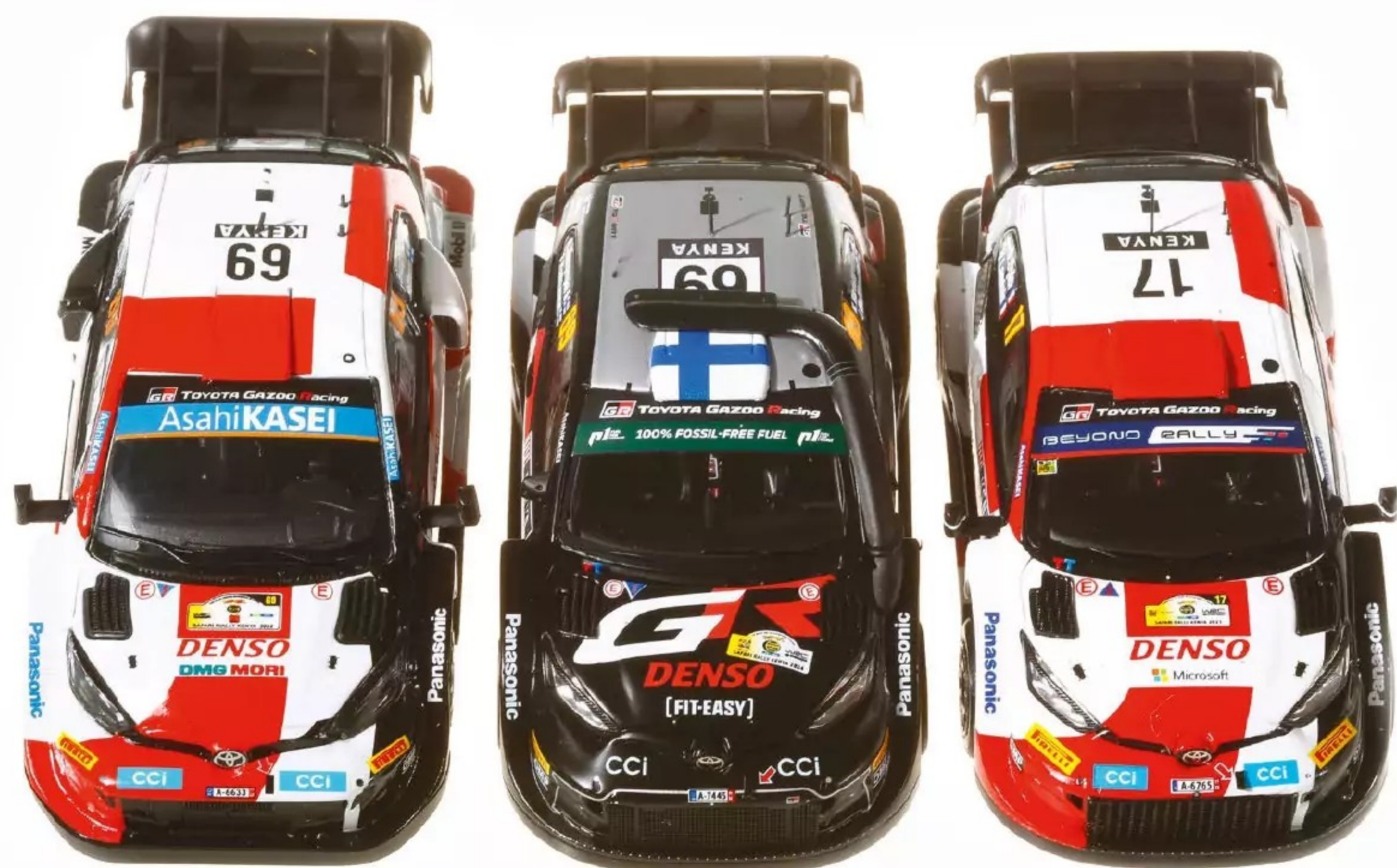
ABOVE Three of the five consecutive wins by Toyota, between 2021 and 2025. The black one in the middle features a special snorkel for the engine's air intake not to inhale water or dust.
