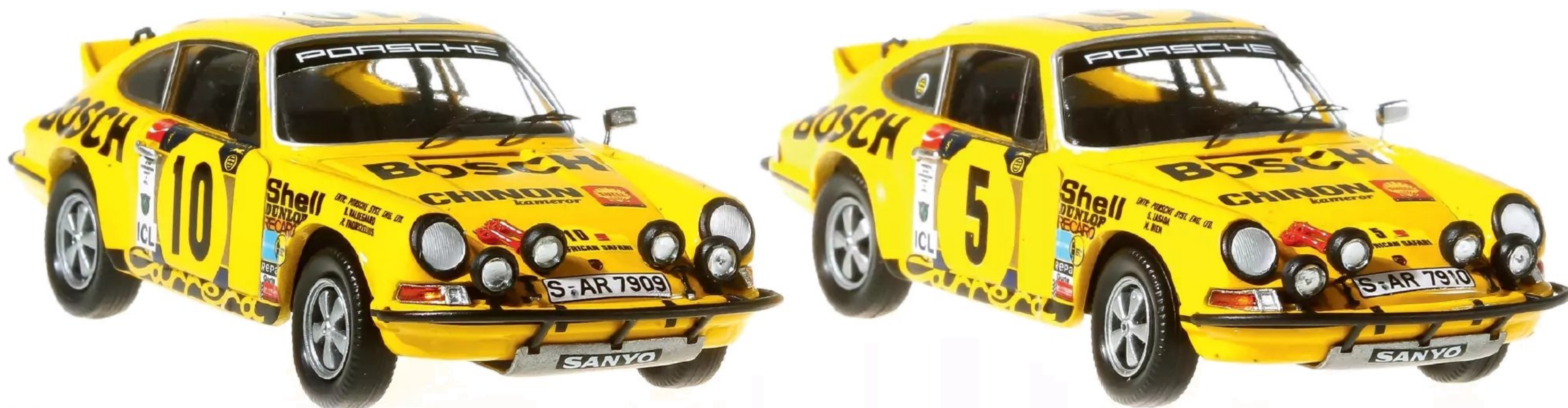
ABOVE The Porsche armada for the 1973 Safari Rally entered this pair of gorgeous yellow 911 RS, sponsored by Bosch. Note the increased ride height, extra spotlights and underfloor protection.
