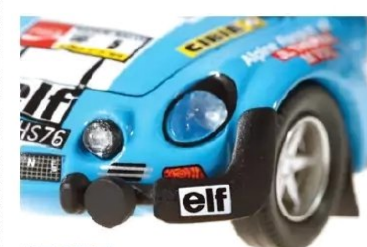
ABOVE Alpine-Renault had extra mud-flaps ahead of the front wheels, to protect the headlights while crossing small rivers.
