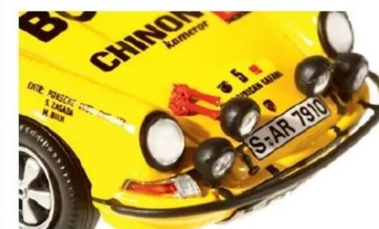
ABOVE Extra spotlights are a must for the Safari, not only for the driver to see, but also for the car to be seen at distance.
