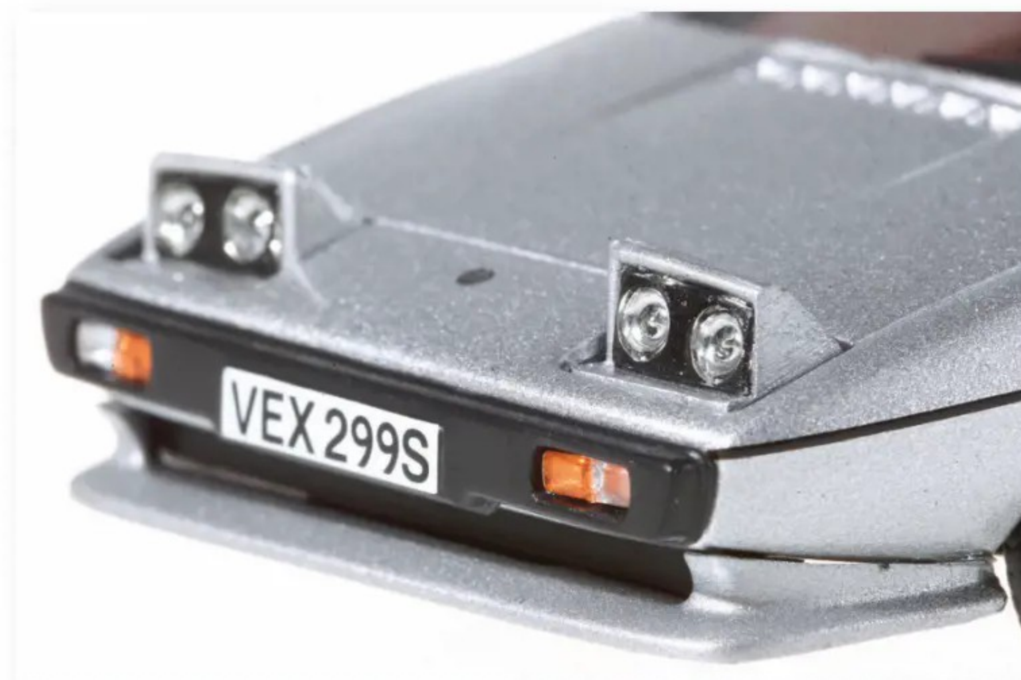
RIGHT Corgi Vanguards' model has moveable headlights that can be easily operated via a small rod under the front.
