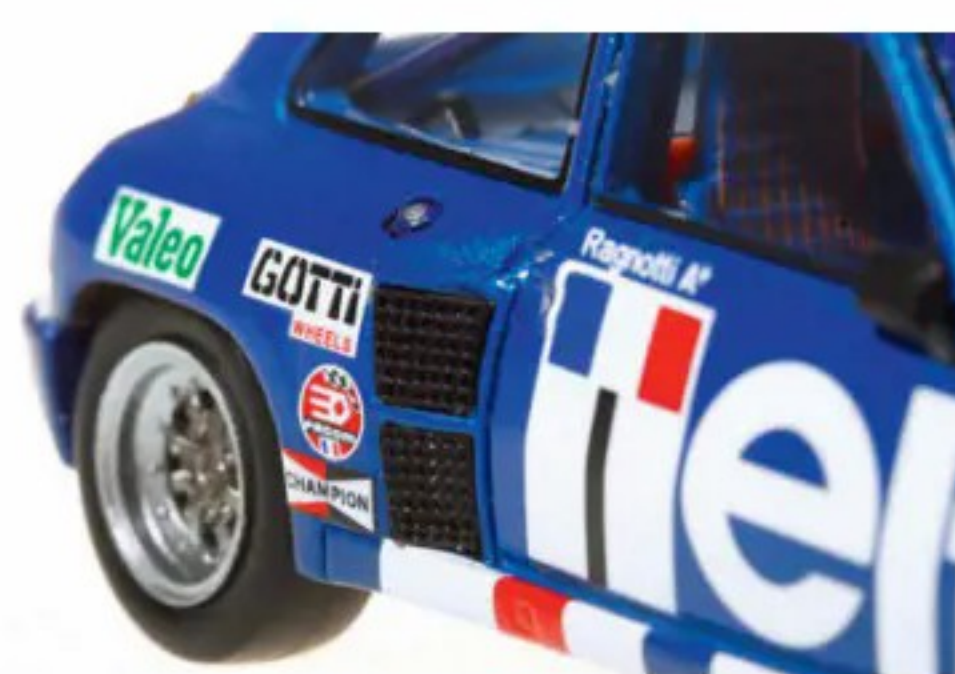
ABOVE Wider rear track needed to accommodate mid-engine and air scoops.
