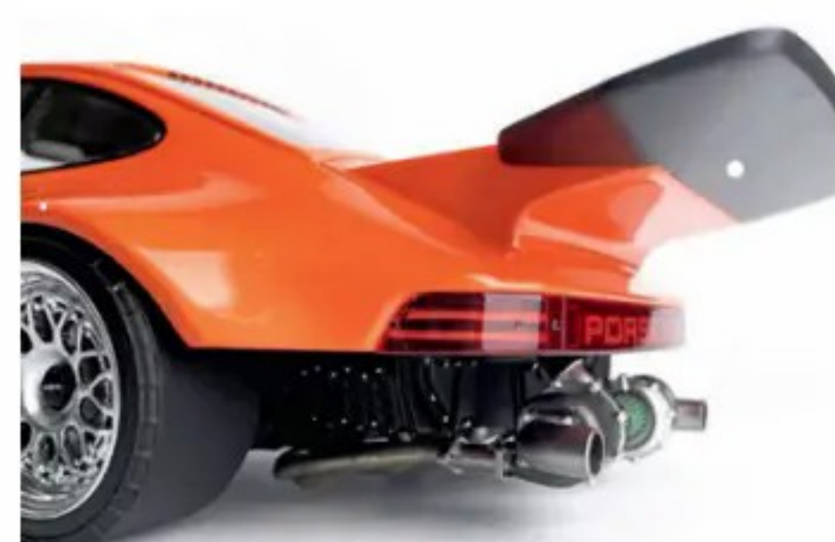
ABOVE The reflector plate is infused with LEDs so that the black PORSCHE lettering of the original is now replaced by illuminated lettering.
