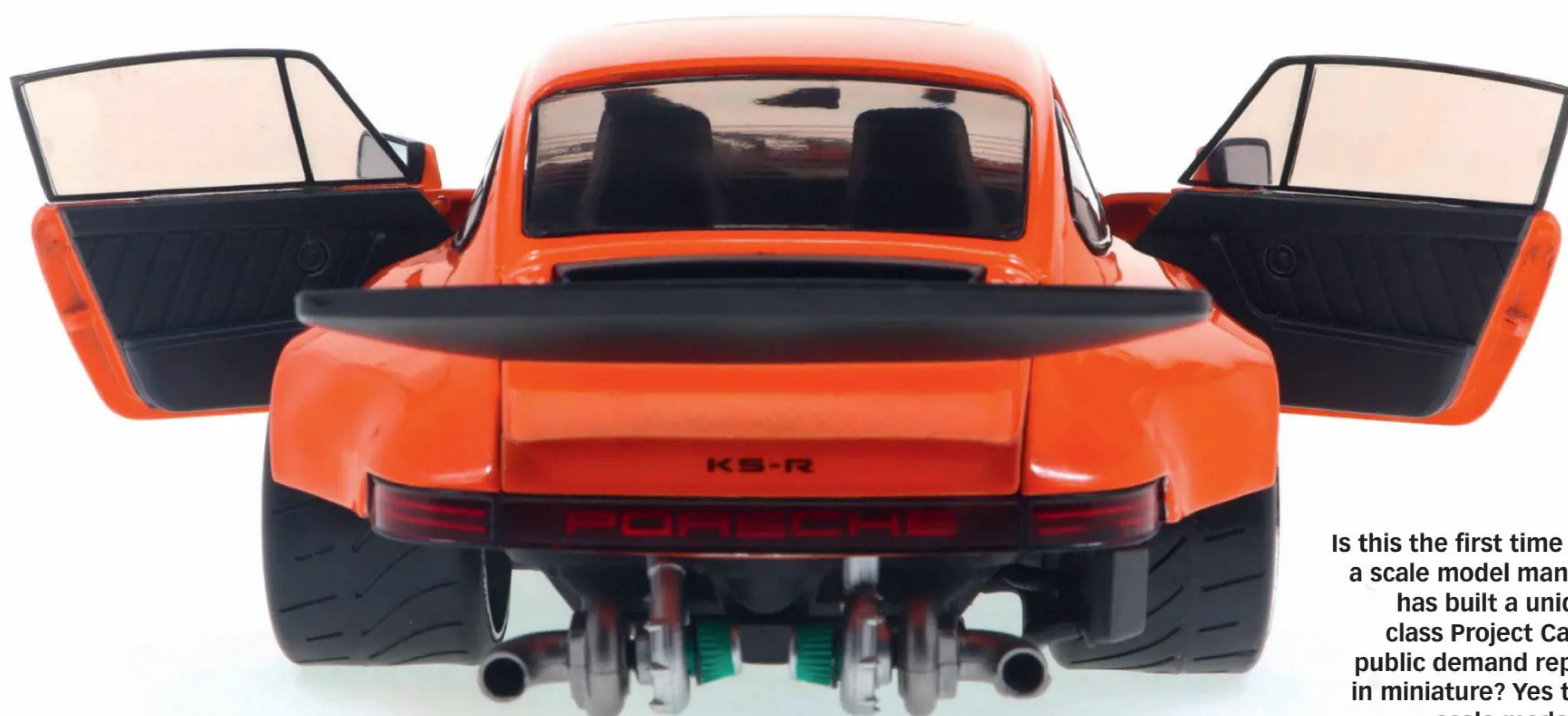
ABOVE The reflector plate is infused with LEDs so that the black PORSCHE lettering of the original is now replaced by illuminated lettering.
