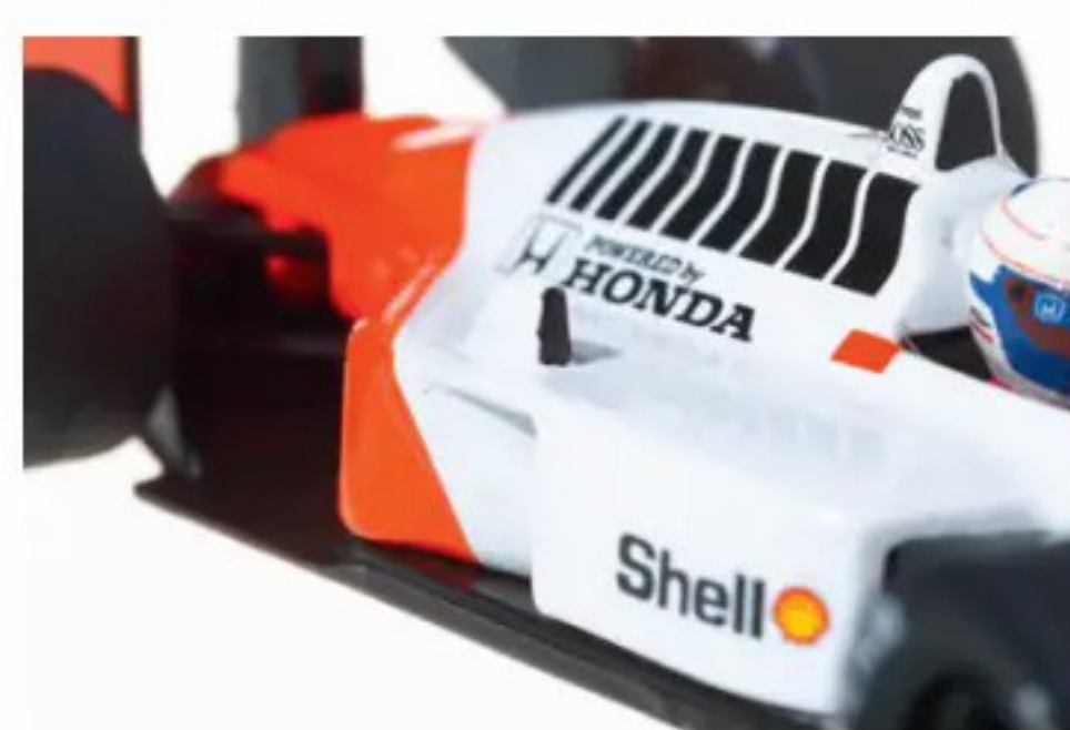
ABOVE Side pods on McLaren's MP4/5B feature a pair of periscope air scoops.
