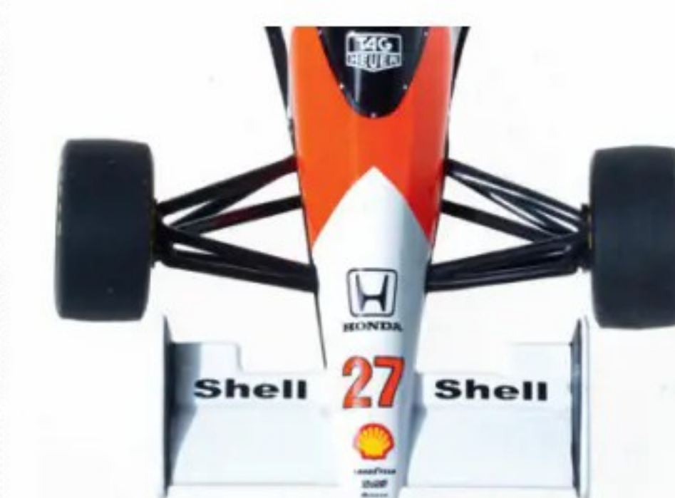
ABOVE Detailed front suspension and front wing in MP4/5B.
