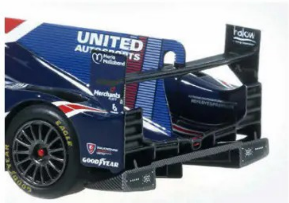
ABOVE Swan neck mount for the rear wing to free aerodynamics beneath it.
