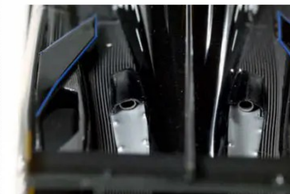
ABOVE Exhaust pipes and heat protectors on Cadillac’s engine cover.
