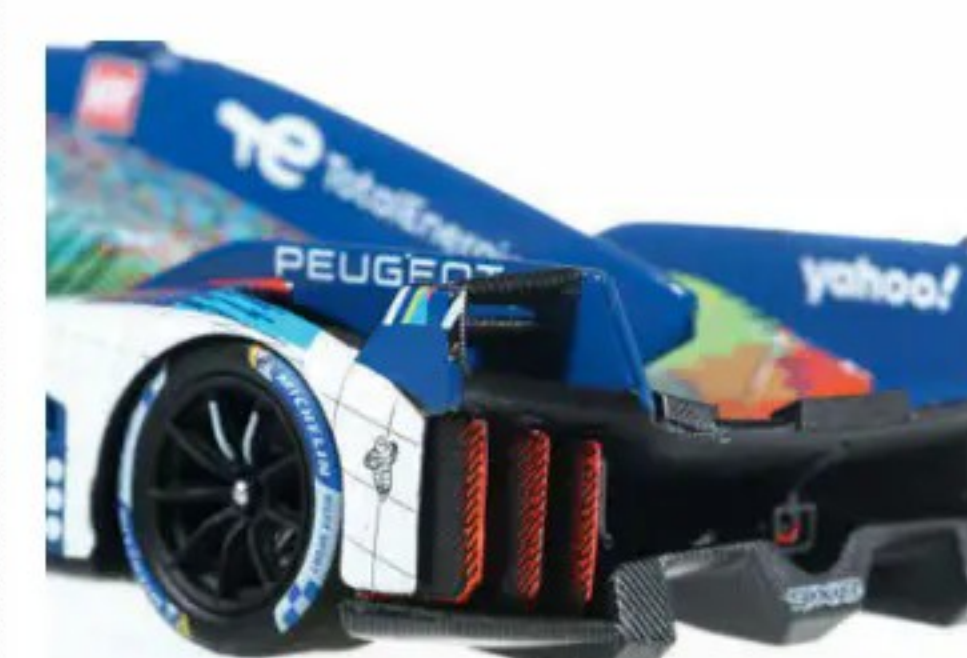
ABOVE Peugeot 9X8 did without a traditional high rear wing, taking downforce from ground effects.
