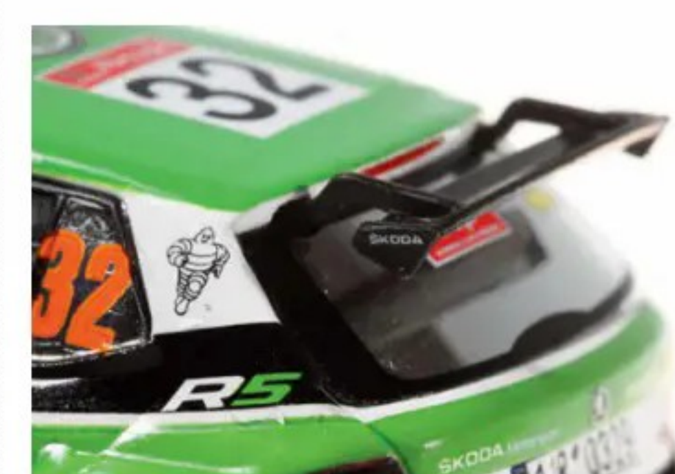
ABOVE Regulations dictate the size and shape of the rear wing in Rally2 specification rally cars.
