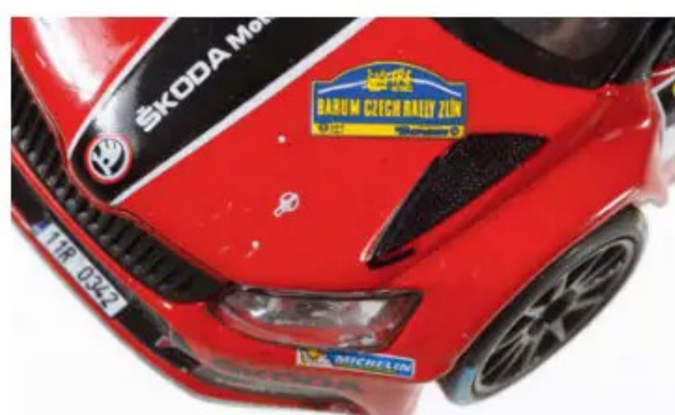
ABOVE Note air duct on the front bonnet, to allow hot air out of the front of the engine compartment.
