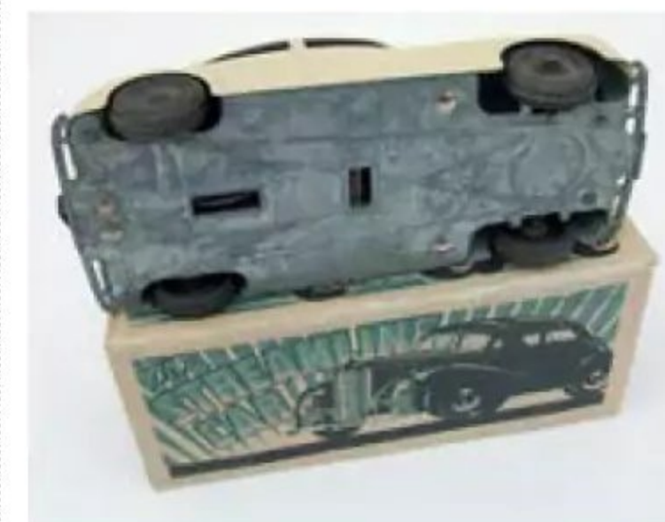
ABOVE Underside of the Castoys saloon car, showing the adjustable front axle and the gears of the mechanism transmitting power to the back wheels.
