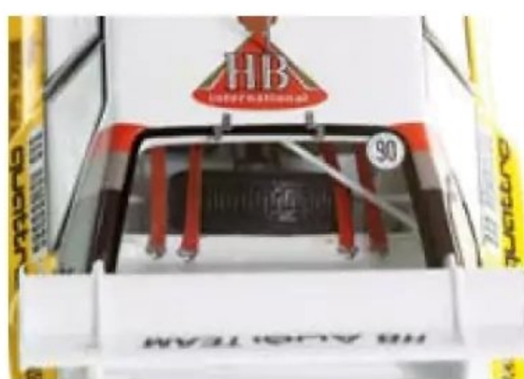
ABOVE Rear window could be opened to extract the spare wheel. Seat belts anchored to the roll cage.
