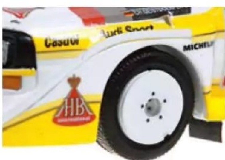
ABOVE For tarmac stages of 1986 rally Portugal, Audi developed these brake heat extractors.
