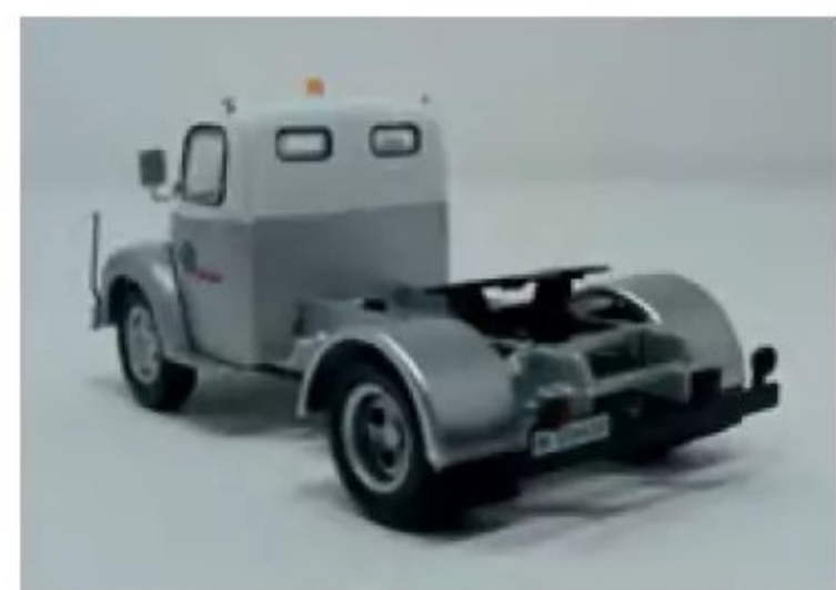
ABOVE ...and its rear, showing the simple coupling plate.
