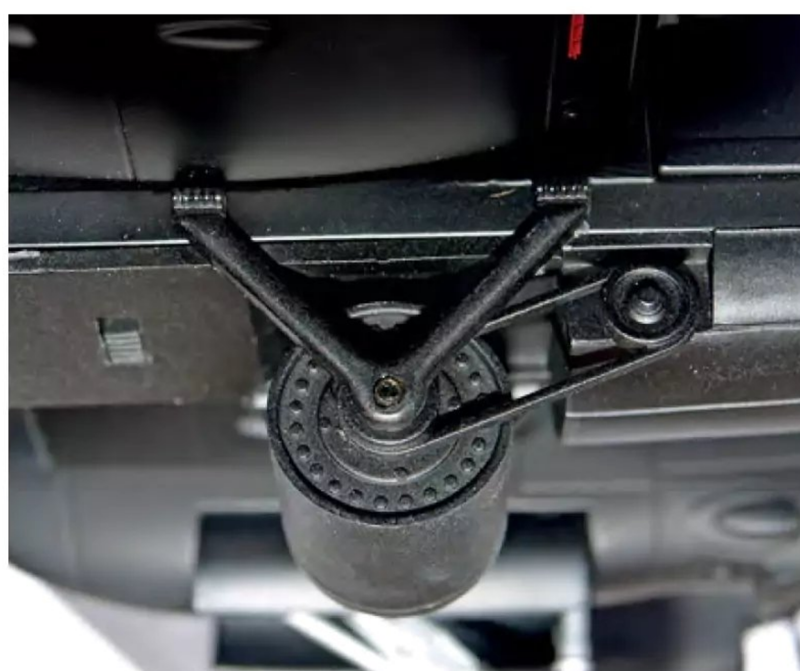
FAR LEFT This view shows the front lamp on the model. Note also the screw which is undone to remove the cover of the Lithium battery.
