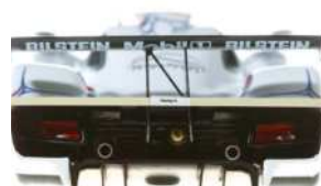
▲ The rear of the 1998 version had a much more developed aerodynamic package, including a new diffuser.
