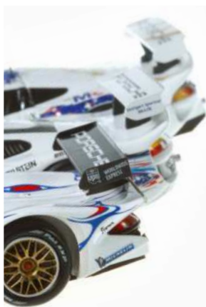
▲ A comparison, side-on, of the evolution of the tail design across the three generations: 1996 at the rear, 1997 in the middle and 1998 to the fore.
