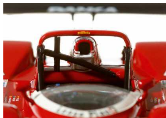
▲ Aerodynamic roll-bar on the 333 SP had hints of the old 250 P in its styling. The air box to the engine was positioned beneath.
