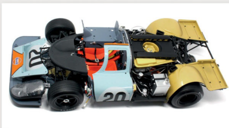
▲ Lots of progress since the last update – we now have some underflooring, more side panels, detailed fuel cell and the two inner rear wheel arches.
