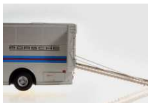
▲ The pair of ramps is held in place by two rods, which can be repositioned to suit.
